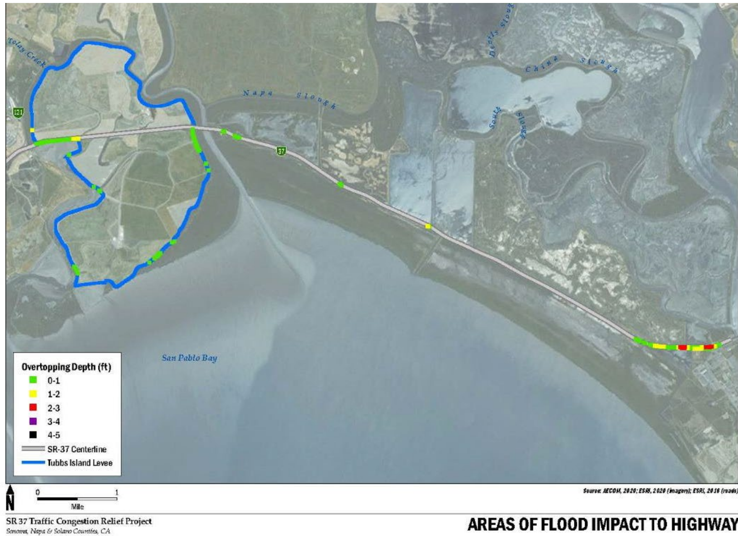
Figure 3-13 Areas of Flood Impact to Highway Under 1.9 Feet of SLR Conditions with a 1-Year Storm Scenario
