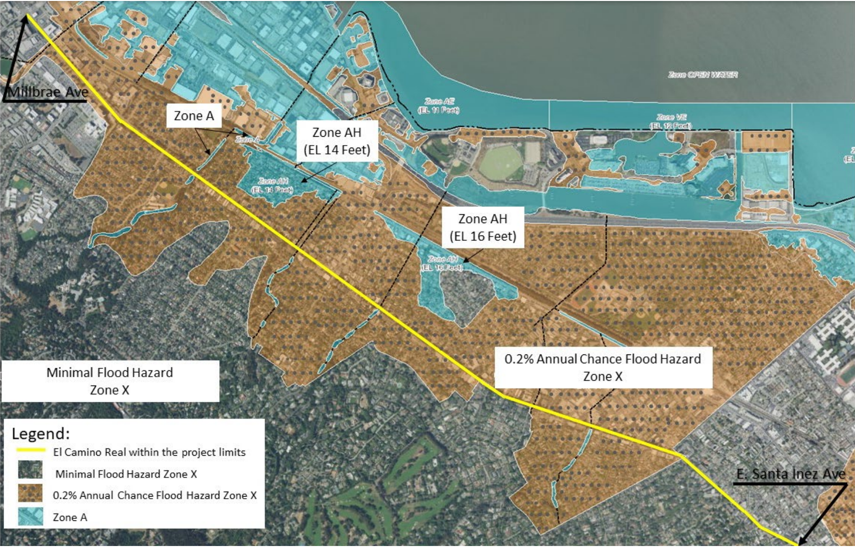
Figure 3.2.1-1: Flood Hazard Zones within the Project Limits
