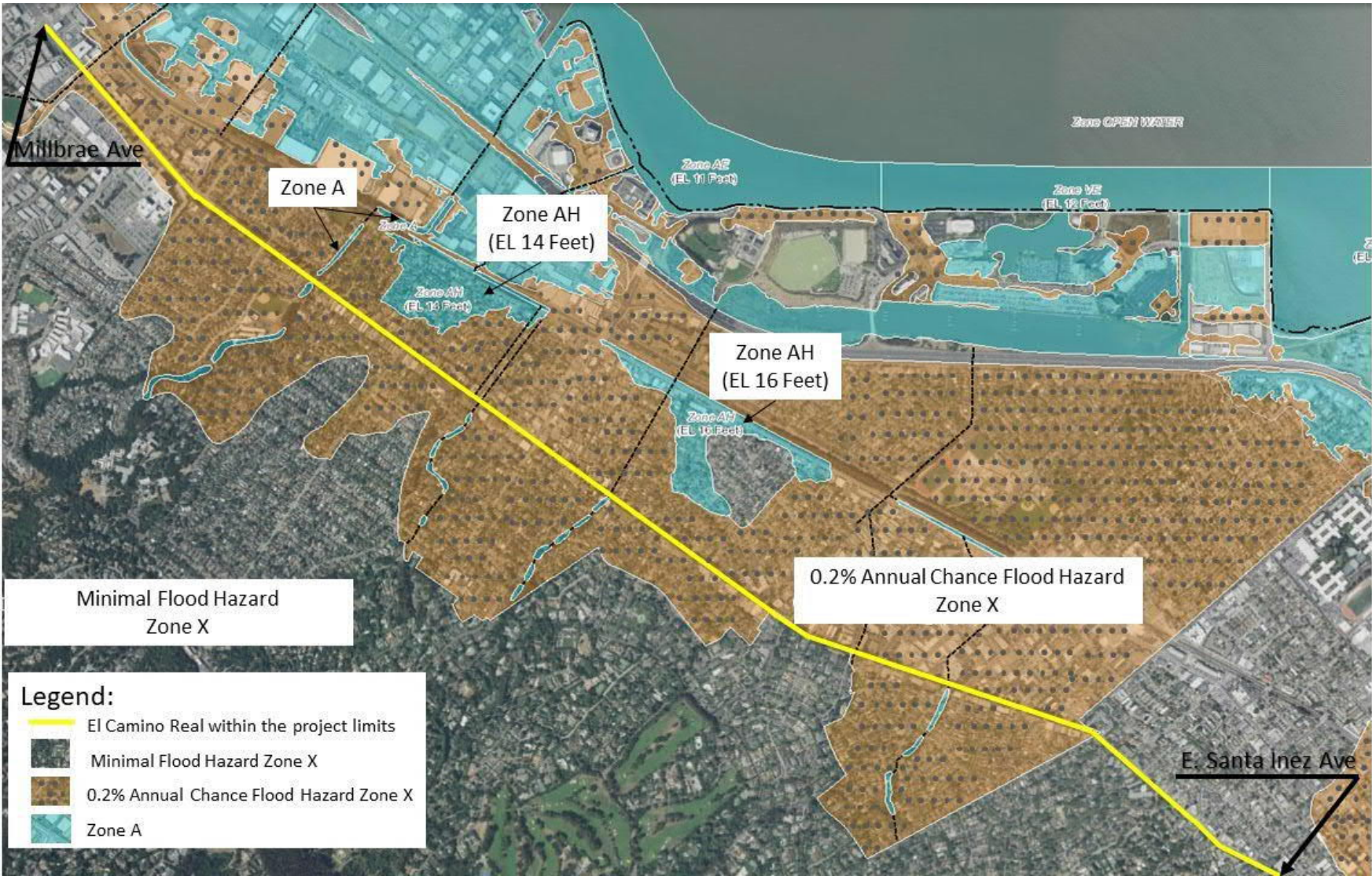
Figure 3.2.1-1: Flood Hazard Zones within the Project Limits
