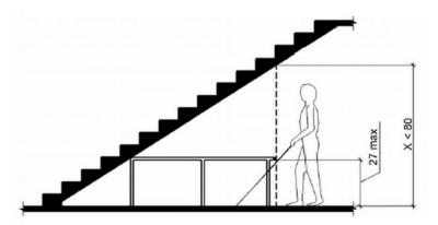
(obtuse angle approach), it is not cane detectable in the opposite direction (acute angle approach) and needs a barrier such as a guy brace, sidewalk guy or similar device for protection from an overhanging obstruction. Discuss these types of situations with your designer. [Inspection Report – Field Verify] {DIB 82-06 4.3.19(2)}
