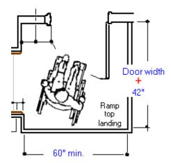
☐ A 2 inch minimum curb or barrier is required along the ramp length.\* {DIB 82-06 4.3.12}
