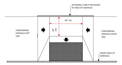
□ Gutter/roadway counter slopes (parallel with predominate pedestrian travel) within 24 inches of the curb ramp not to exceed 5.0 percent (see below). [Inspection Report – Field Measurement] {DIB 82-06 4.3.8(4)}
