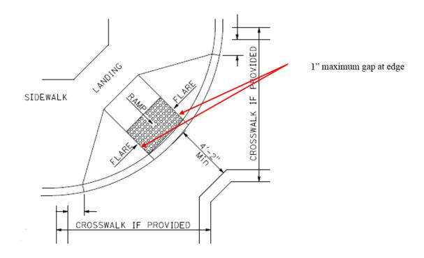
□ Placement of DWS on radial curb ramps such as a blended transition should be addressed with a construction detail in the project plans. If not provided, discuss with your designer.
