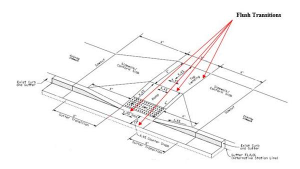
□ Curb ramp flare slope not to exceed 10.0 percent, measured at back of curb (see below). [Inspection Report – Field Measurement] {DIB 82-06 4.3.8(5)}
