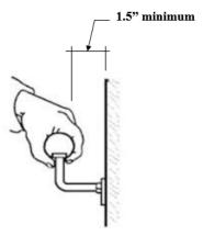
☐ Handrails shall not rotate within their fittings. {DIB 82-06 4.3.10(6)}
