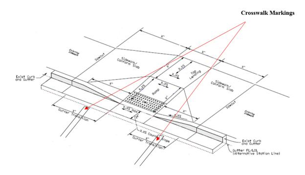
□ Diagonal curb ramps with flared sides such as those shown on RSP A88A – Detail B "Typical One-Ramp Corner Installation" must provide a minimum of 2 feet of curb on each side of curb ramp within the limits of crosswalk if provided. Diagonal curb ramps must also provide a 48 inch minimum clear space within the markings of a marked crossing. Note that the standard plan shows a conservative 50 inch dimension (see next page). [Inspection Report – Field Verify] {DIB 82-06 4.3.8(6) & (7)}
