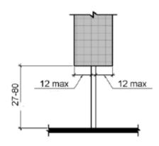
□ If a sign or other obstruction is mounted between posts or pylons and the clear distance between posts or pylons is greater than 12 inches, the lowest edge of such sign or obstruction shall be either 27 inches or less or 80 inches or more from the surface. [Inspection Report – Field Verify] {DIB 82-06 4.3.19(3)}
