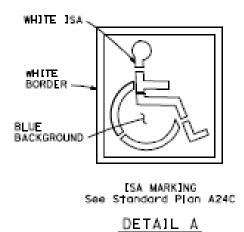
☐ For off-street accessible parking stalls, include the International Symbol of Accessibility (ISA) marking (see Standard Plans A90A and A24C) with white border, blue background and white ISA. Place in each accessible parking stall at the rear limit and centered in the width of the stall. [Inspection Report – Verify] {DIB 82-06 4.3.17 and Standard Plan A90A}
