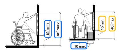
□ Obstructed high side reach − Where a clear floor or ground space allows a parallel approach to an element and the high side reach over an obstruction, the height of the obstruction shall be 34 inches maximum and the depth of the obstruction shall be 24 inches maximum. The high side reach shall be 48 inches maximum for a depth of 10 inches maximum. Where the depth exceeds 10 inches, the high side reach shall be 46 inches maximum for a reach depth of 24 inches maximum. {DIB 82-06 4.3.15(3)}
