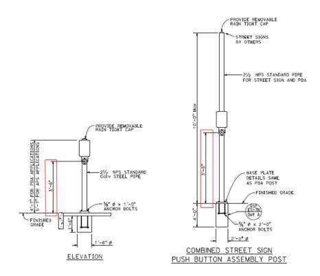
$\Box$  Face of the PPB is to be mounted parallel to the crosswalk direction it serves. {*CA-MUTCD* – Section 4E.08 04-E}
