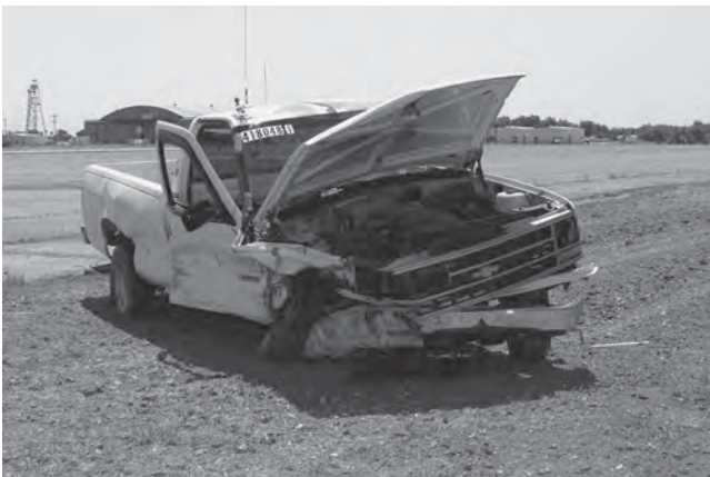
Figure 43. Pickup truck after impact with Texas T411 bridge rail.
