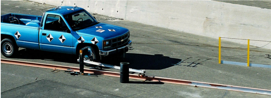
Figure 7-1 – Typical guidearm release
