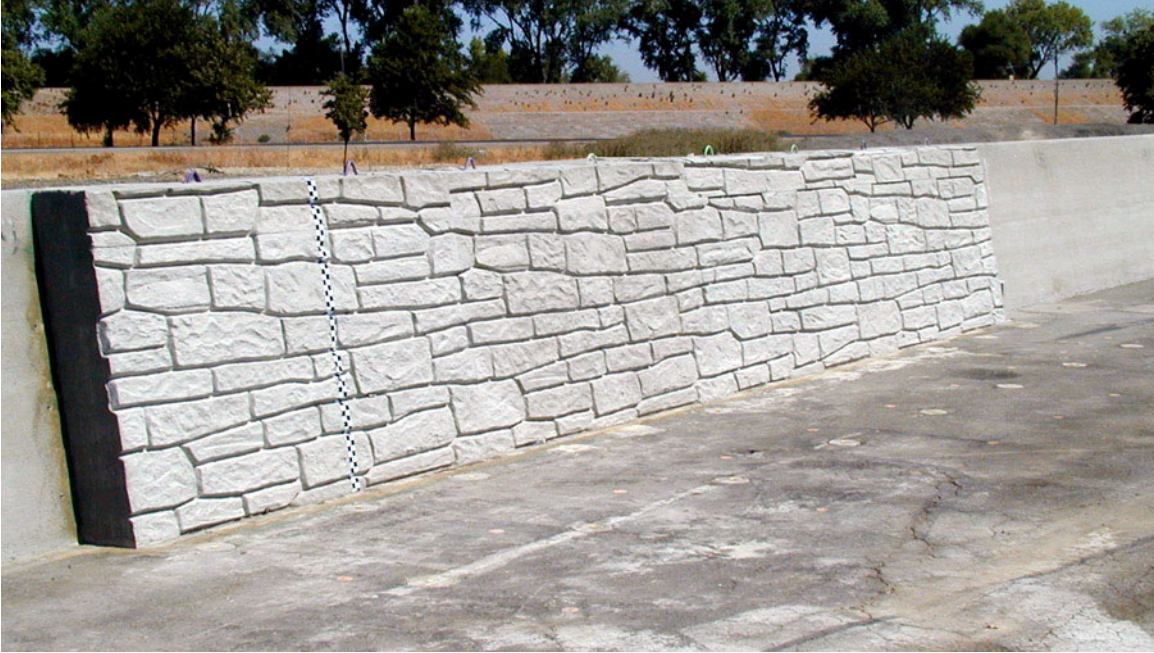
Figure 2-43 Drystack test article prior to Test 587
