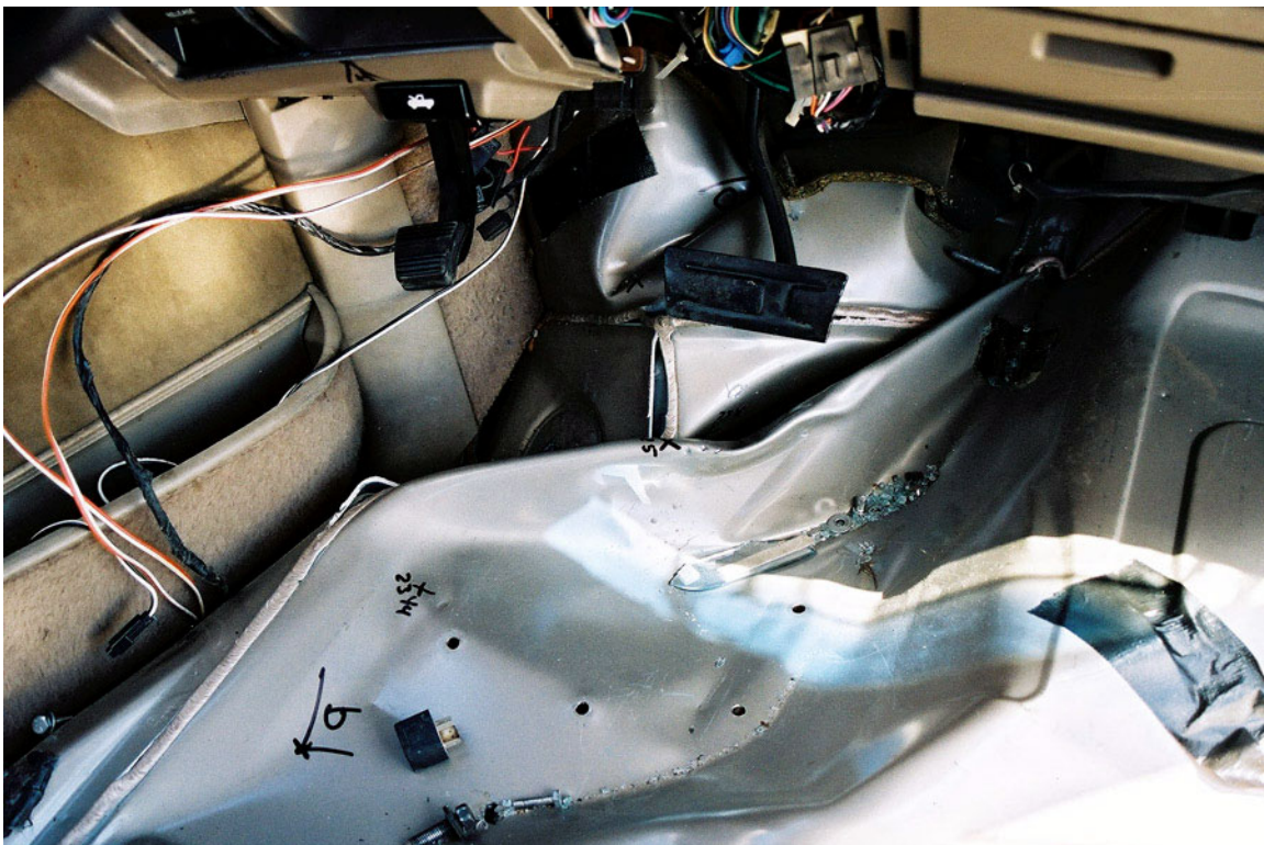
Figure 2-24 Vehicle floorboard deformation after Test 583
