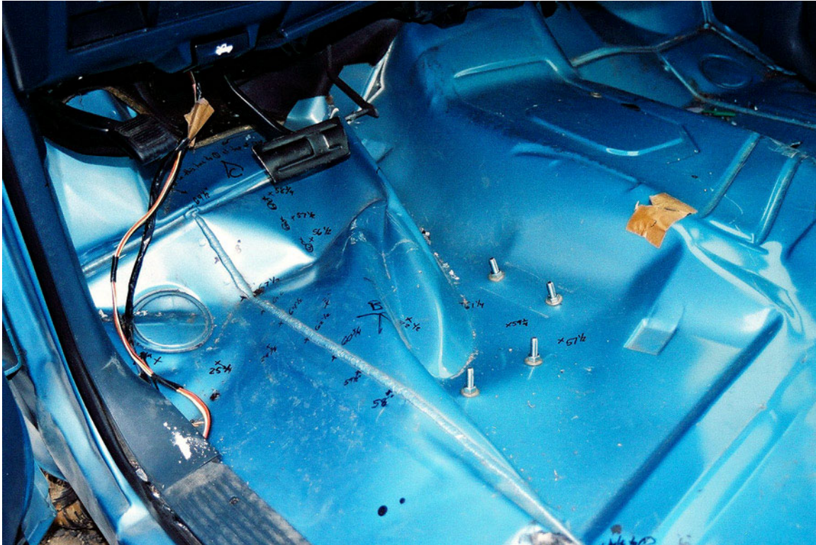
Figure 2-55 Vehicle floorboard after Test 588
