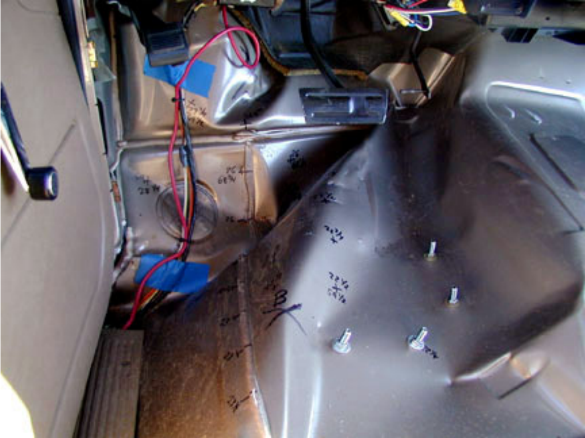
Figure 2-63 Vehicle floorboard after Test 589
