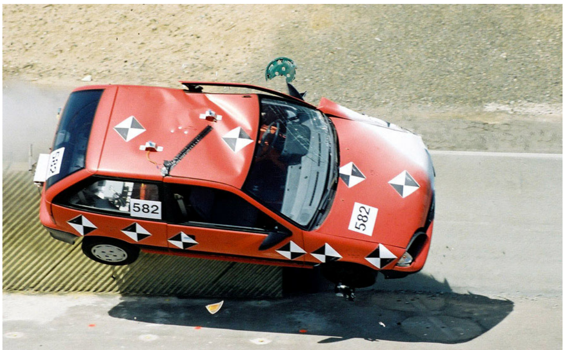
Figure 2-12 Test vehicle 582 during the Test (the vehicle rolled over twice to the left after landing)
