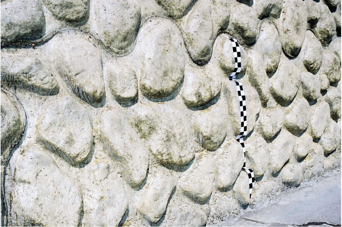
Figure 2-7 Cobble pattern test article prior to Test 581
