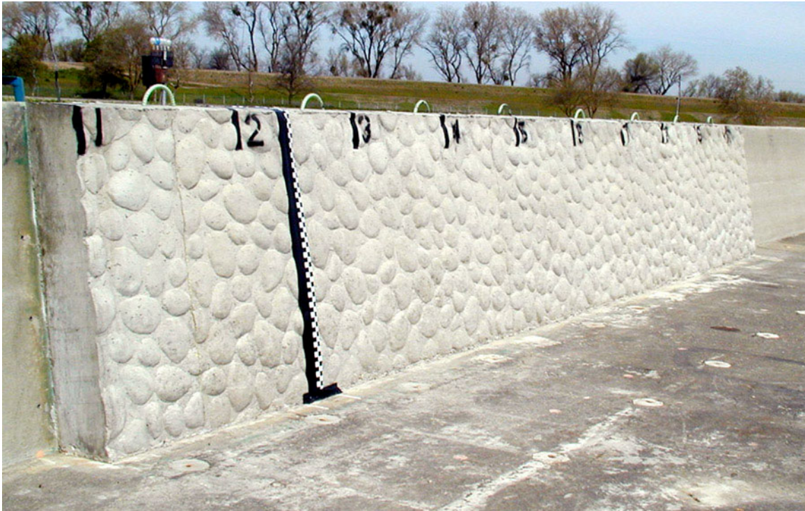
Figure 2-59 Shallow cobblestone test article prior to Test 589
