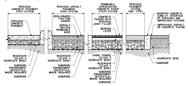
Figure 8-J – Example Pervious Pavement Treatment BMP
