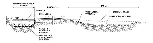
Figure 8-I – Example Detention Basin Treatment BMP
