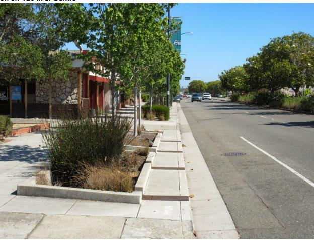
Figure 8-N - Warning curbs surround bioretention planters adjacent to on-street parking on SR-123 in El Cerrito
