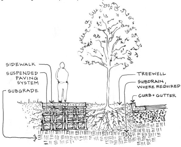
Figure 8-E – Diagram of a structural soil system
