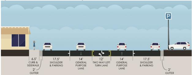
Existing pedestrian facilities are discontinuous, and bicycle facilities are absent. The wide shoulders and parking lanes in this cross section present an opportunity to provide separated facilities for bicycle and pedestrian users. The presence of abundant off-street parking further supports the elimination or reduction of on-street parking in the roadway cross section.
