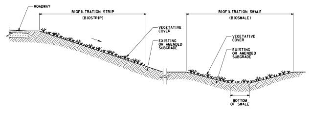
Figure 8-H – Example Design Pollution Prevention Infiltration Area Treatment BMP
