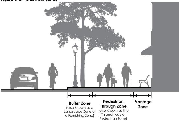
While these zones may not be clearly demarcated, and in fact in some cases concrete pavement runs continuously from back of curb to face of building, these zones are conceptually useful to plan for a pedestrian facility that meets all users' needs. An example of a sidewalk exhibiting these three zones is shown in Figure 5-P.
