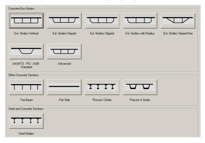
Figure 4.2-17 Various Bridge Sections
