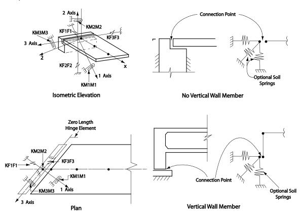
Figure 4.2-11 Foundation Spring Definition
