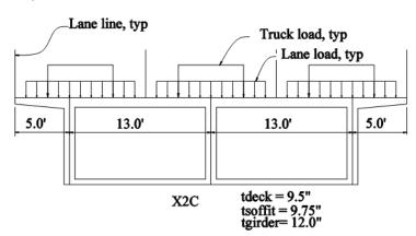
Figure 4.4-6 Live Load Distribution For Two-Cell Box Girders Snapshot In Group 4
