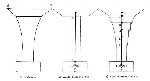
Figure 4.2-5 Single-Column Bent Models (Priestley et al, 1996)
