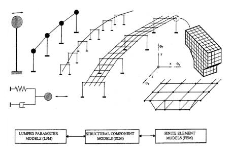
Figure 4.2-3 Levels of Modeling for Seismic Analysis of Bridge (Priestley, et al 1996)
