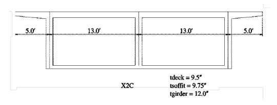
Figure 4.4-2 Live Load Distribution For Two-Cell Box Girders Snapshot
