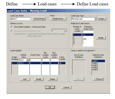
Figure 4.4-11 Analysis Cases Snapshot in One-Lane Loaded
