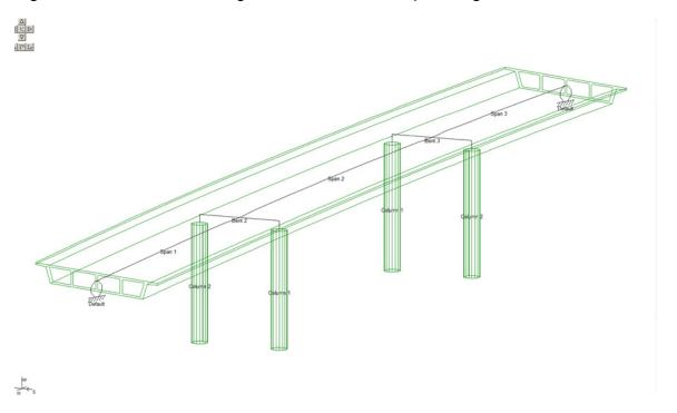
Figure 4.2-14 Example Bridge - CTBridge Model
