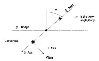
Figure 4.2-9 Foundation Spring Definition at a Bent
