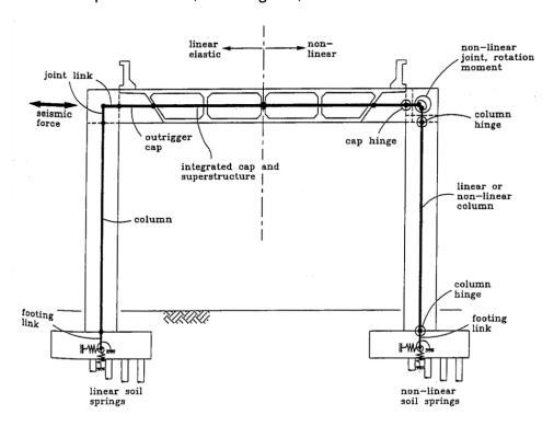
Figure 4.2-8 Multi-Column Bent Model (Priestley et al, 1996)
