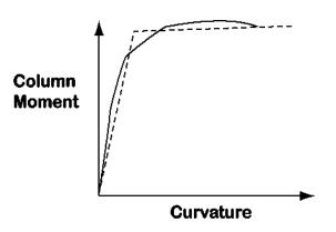
Figure 4.3-3 Typical Moment-Curvature Curve for a Concrete Column
