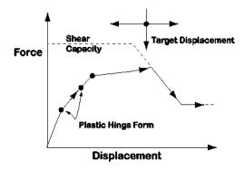
Figure 4.3-2 Typical Force Displacement Curve for a Concrete Column
