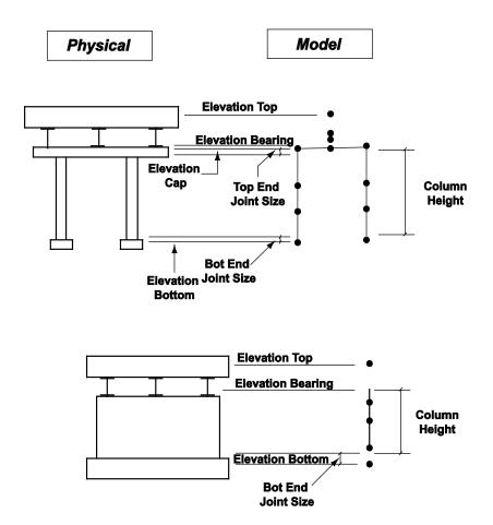
Figure 4.2-6 Superstructure-Bent Connection
