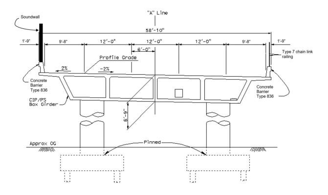
Figure 4.2-13b Typical Section View of Example Bridge
