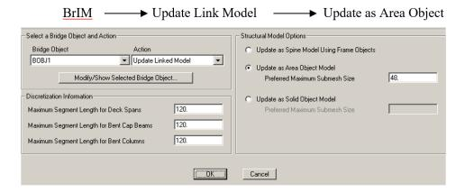
Figure 4.4-7 Bridge Modeler Snapshot
