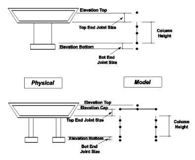
Figure 4.2-2 Model Discretization for Monolithic Connection
