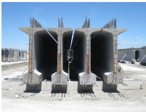
A) Pretensioned bulb-tee girders
