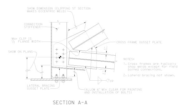
Figure 11.5.1 Cross Frames with Lateral Bracing
