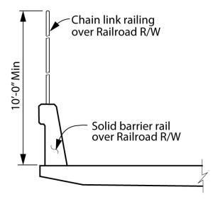
Figure 12A.A.2 Typical Fence on Barrier Detail
