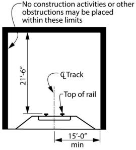
Figure 12A.A.3 Minimum Construction Clearance Envelope
