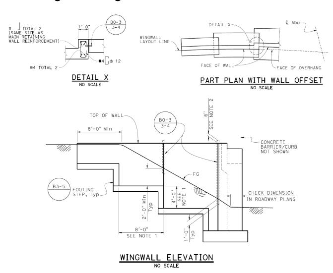
Figure 6.10.1 Retaining Wall Wingwalls
