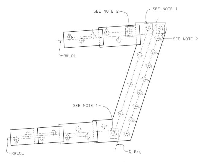
Figure 6.5.1 Piles at Abutment Corners
