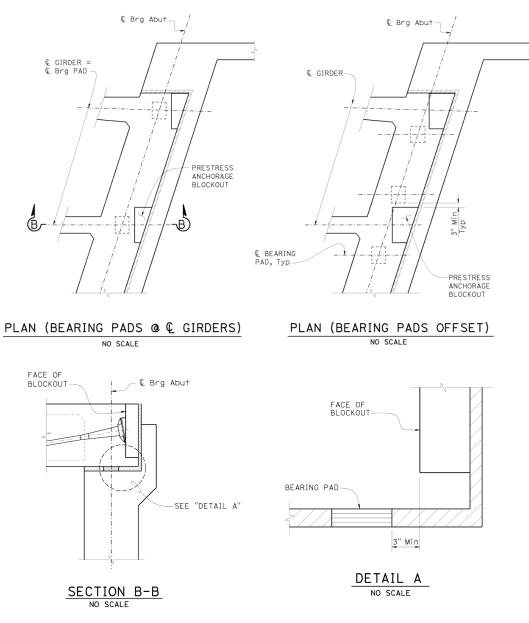
Figure 6.6.1 Bearing Pad Location at Anchorage Blockout
