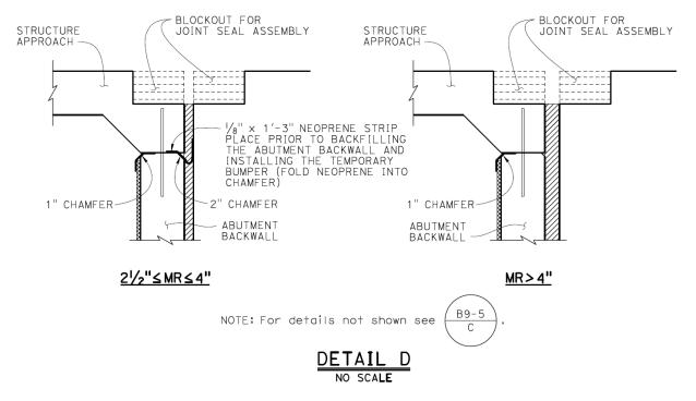
Figure 6.7.3 Joint Seal Protection Detail (MR > 2½")
