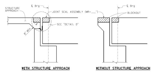
Figure 6.7.2 Joint Seal Assemblies (MR >  $2\frac{1}{2}$ ")
