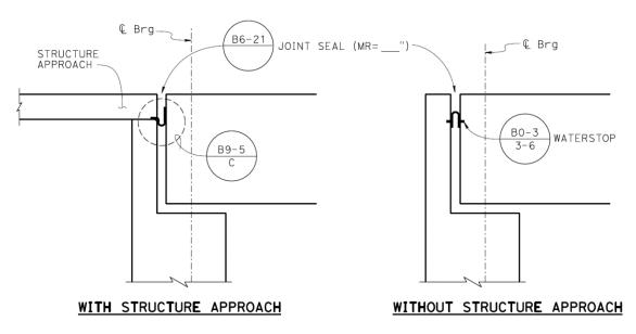
Figure 6.7.1 Sealed Joints (MR ≤ 2")
