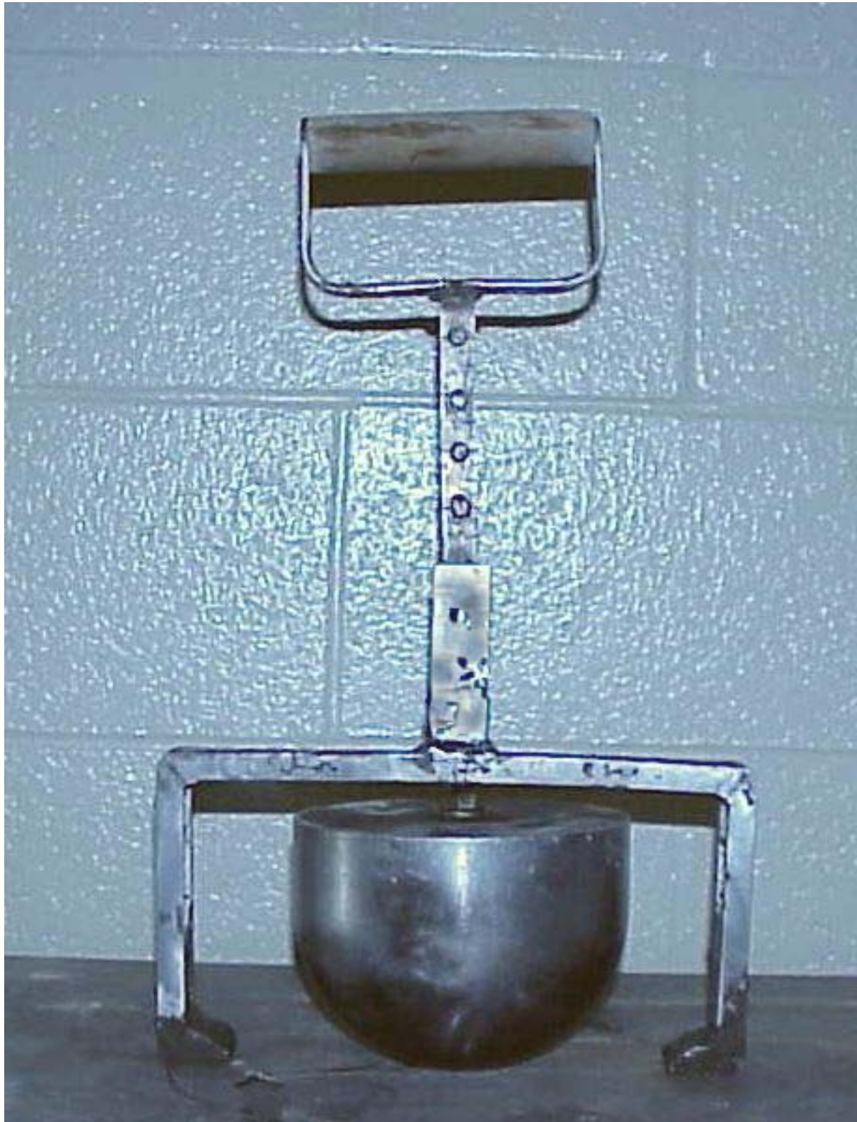
FIGURE 1. Ball on Table Showing Condition at Zero Penetration
