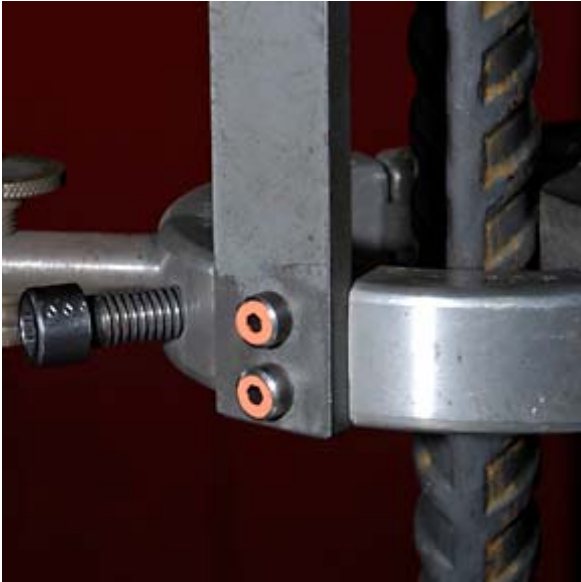
Figure 1b. Close up of hex socket bolts used to hold the vertical bars during the set up of the measuring device.
