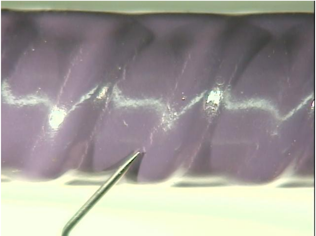
Figure 5. Test sample showing discoloration in coating after the bend test. This type of discoloration is due to stretching of the coating during bending and is typical. Discoloration of the coating after bending does not constitute a failure of the bend test.
