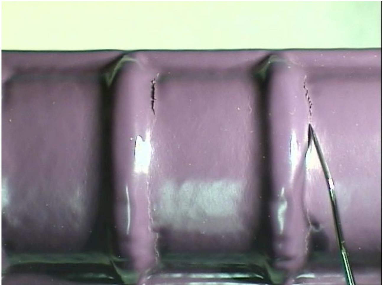
Figure 3 Test bar showing two of three breaks in the epoxy coating at the outer bend radius of a test bar. The breaks appear to be cracks that expose the underlying metal. Exposed underlying metal can be confirmed, if needed, by viewing with a 10X-magnification device.
