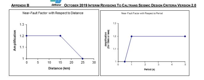
**Figure B.1** Near-Fault adjustment factor as a function of distance and spectral period. The distance measure is based on the closest distance to any point on the fault plane
