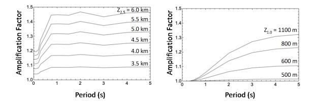
**Figure B.2** Basin amplification factors for the Campbell-Bozorgnia (2014) and Chiou-Youngs (2014) ground motion prediction equations. Chiou-Youngs is  $V_{S30}$  dependent. Plotted are basin amplification factors for  $V_{S30}$  = 259 m/s.
