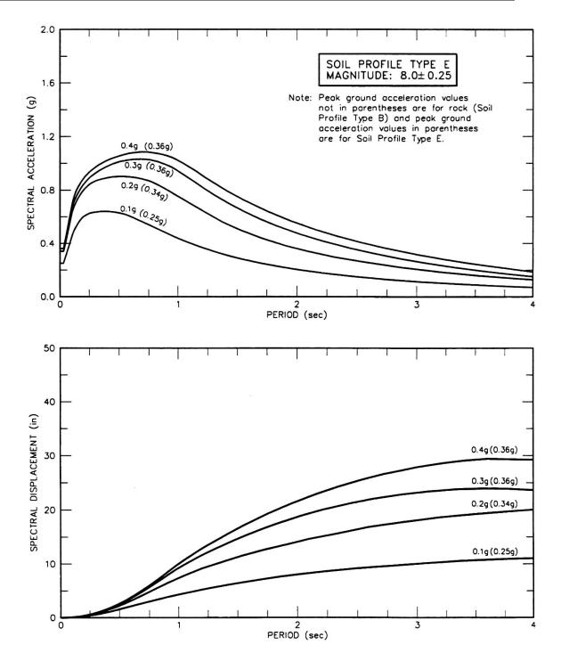
**Figure B.13** Spectral Acceleration and Displacement for Soil Profile E ( $M = 8.0 \pm 0.25$ )
