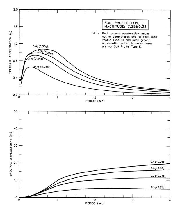
**Figure B.12** Spectral Acceleration and Displacement for Soil Profile E ( $M = 7.25 \pm 0.25$ )
