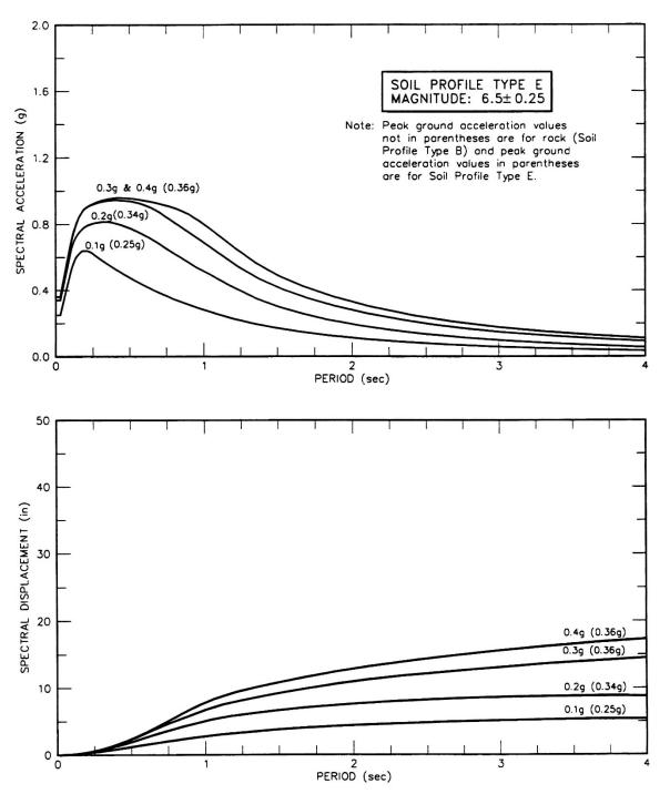
**Figure B.11** Spectral Acceleration and Displacement for Soil Profile E ( $M = 6.5 \pm 0.25$ )
