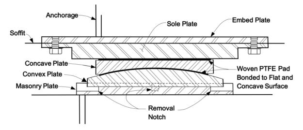
Figure 14.1.5.1 Example of Multidirectional Sliding PTFE Spherical Bearing with Replaceable Sliding Surfaces
