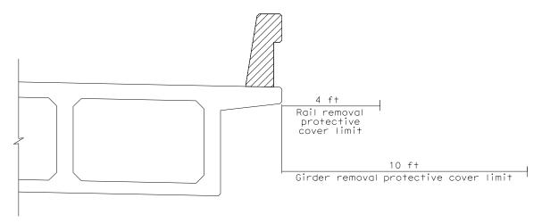
Figure 5-6. Protective Cover Minimum Limits
