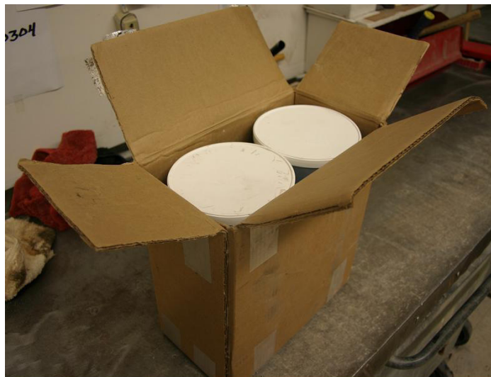
Figure 9-4. Shipping Test Cylinders.
