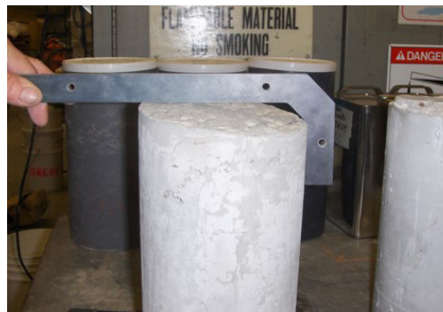
(e) Cylinder Top Not level.
