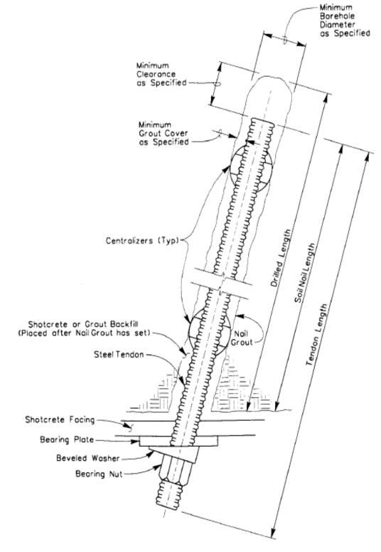
Figure 11-4. Soil Nail Detail.
