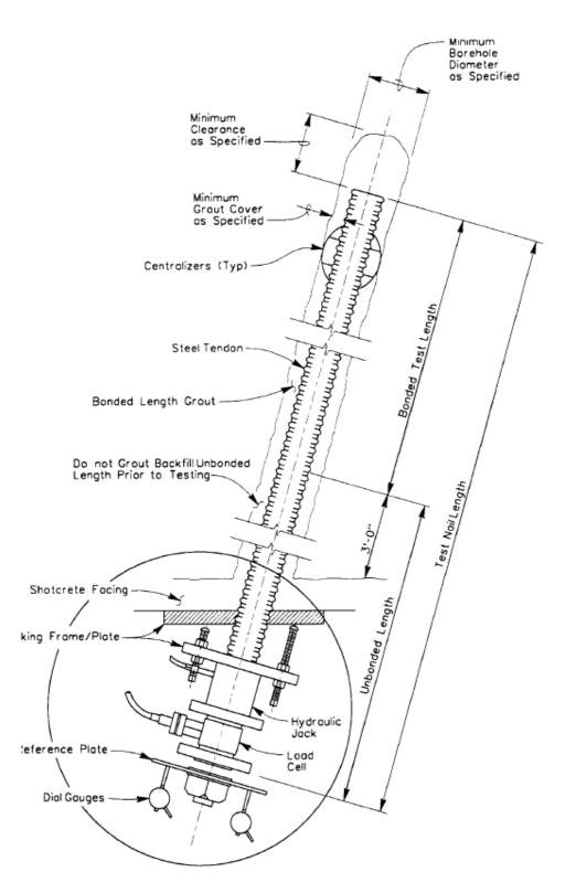
Figure 11-5. Verification/Test Nail Detail.
