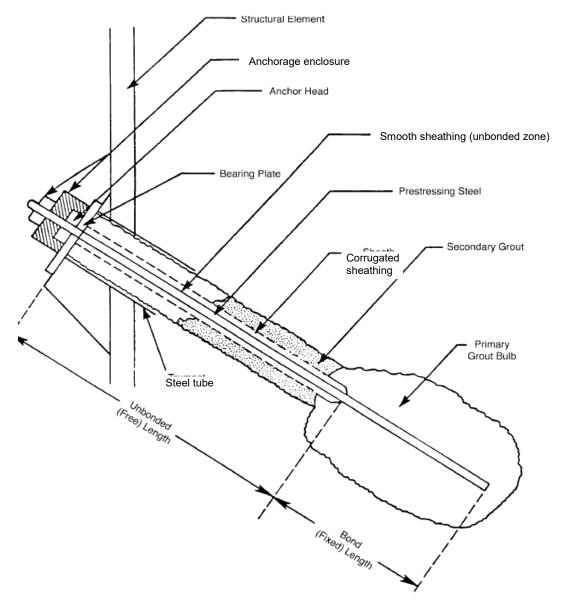
Figure 11-1. Sub Horizontal Ground Anchor Schematic.
