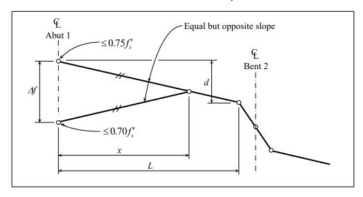
The *Standard Specifications*<sup>56</sup> requires that the maximum temporary tensile strength (jacking stress before anchor set) must not exceed 75% of the specified minimum ultimate tensile strength of the prestressing steel. This initial stress is just after anchor set but before any long term losses occur, such as concrete shrinkage, relaxation of prestress steel, etc.
