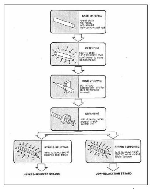
Figure 4-1 – Low-Lax Strand Manufacturing Process.
