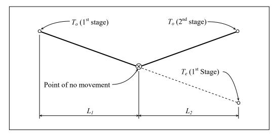
After obtaining the theoretical elongations, the measurable elongations are calculated. This is usually equal to 80% of the calculated elongation (using the actual E and A) from the first end and 100% from stressing the second end.
