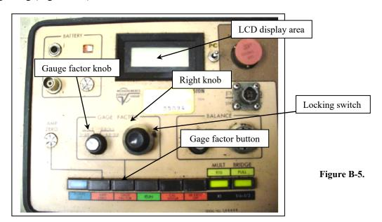
7. Push the "run" button, use the knob on the right in the "balance square" to set the number in the LCD display to "0.000+/-" keeping in mind that this button also has a locking switch. Move the switch counter clockwise to unlock. After adjustment, move the switch to the lock position (clockwise) (Figure B-6).
