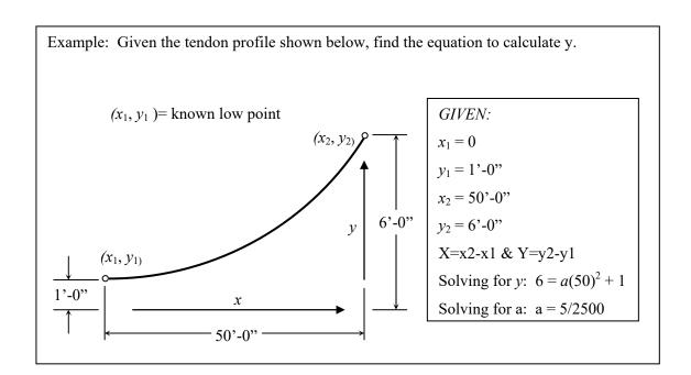
The final check for the duct alignment should be verified by visually observing a smooth tendon path. It is recommended that the taped duct joints be staggered for multiple tendon girders so that a misalignment of the ducts does not occur. Waterproof tape must be used at all duct connections.<sup>11</sup>
