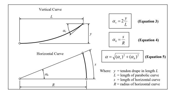
To determine the loss due to friction expressed as a fraction of the temporary jacking stress, use the following formula:
