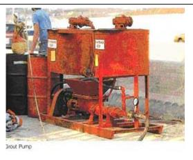
Photo 9-2 – DSI Grout Pump.
