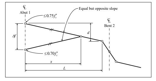
The *Standard Specifications*<sup>56</sup> requires that the maximum temporary tensile strength (jacking stress before anchor set) must not exceed 75% of the specified minimum ultimate tensile strength of the prestressing steel. This initial stress is just after anchor set but before any long term losses occur, such as concrete shrinkage, relaxation of prestress steel, etc.
