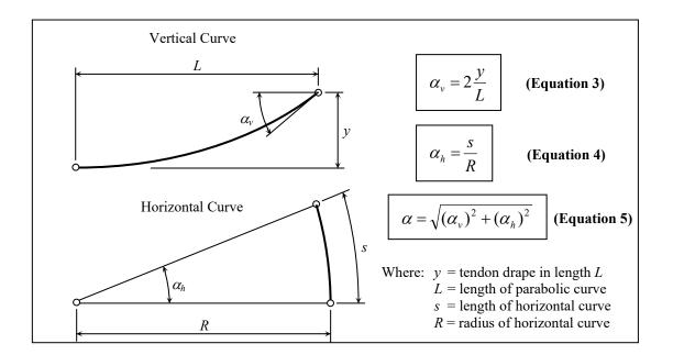
To determine the loss due to friction expressed as a fraction of the temporary jacking stress, use the following formula:
