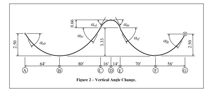
**Step 1**: Tendon elongations during the stressing operation are a function of both the average stress in the strands, and the length of the tendon. The stress in the strands vary along the tendon path due to angular friction between the tendon and the inside surface of the duct. Since there is no horizontal curvature given in this exercise, the angle changes are based on the vertical tendon profile only.
