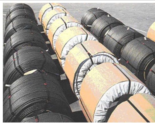
Photo 4-12 – Cal-Wrapped Strand Packs.
