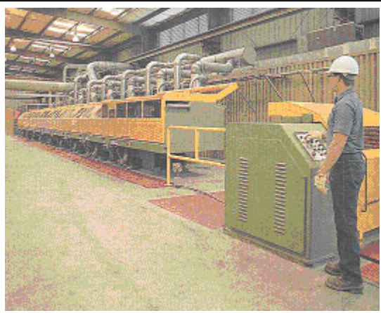
Photo 4-14 – Sumiden Cold-drawing Process.
