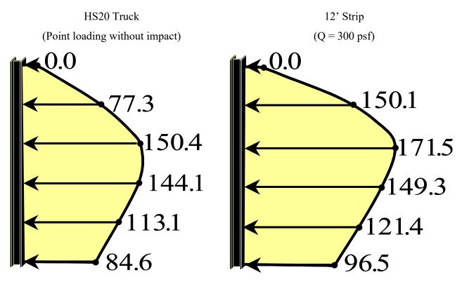
CONCLUSION: Strip load of Q = 300 psf compares favorably to a point load evaluation for HS20 truck loadings.
