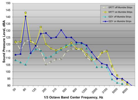
Figure A35:  $\frac{1}{3}$  octave band rear door acceleration spectra for Ford Fusion test vehicle on and off mumble strips with SRTT and Goodyear test tires
