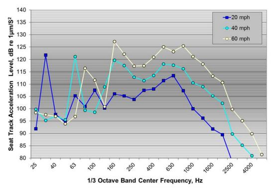
Figure 56:  $\frac{1}{3}$  octave band seat track acceleration level on ground rumble strips for the Malibu test vehicle at 20, 40, and 60 mph
