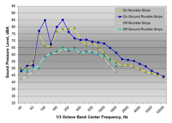
Figure 36:  $\frac{1}{3}$  octave band interior noise spectra for Civic test vehicle on and off mumble strips and ground rumble strips
