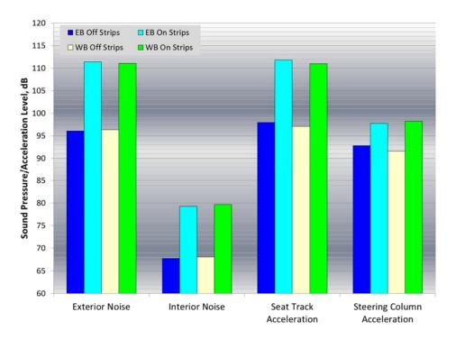
Figure A2: Overall noise and acceleration levels for Expedition test vehicle traveling at 60 mph both on and off ground rumble strips and both eastbound and westbound
