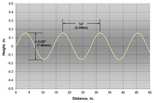
Figure 1: Recommended sinusoidal profile for mumble strips
