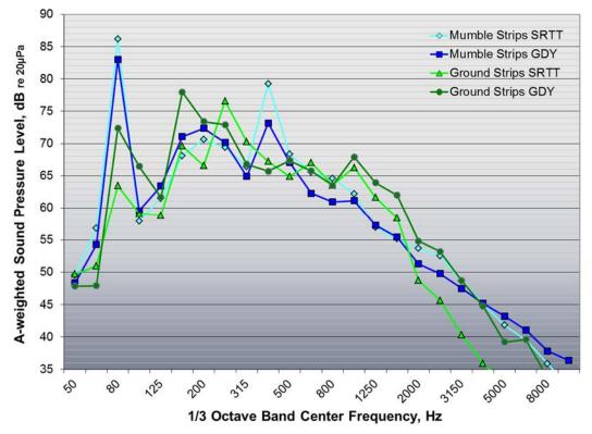
Figure 63: <sup>1</sup>/<sub>3</sub> octave band interior sound pressure levels measured with GDY tires and SRTT
