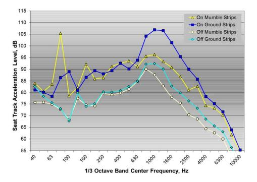
Figure A17:  $\frac{1}{3}$  octave band seat track acceleration spectra for Expedition test vehicle on and off mumble strips and ground rumble strips at 60 mph
