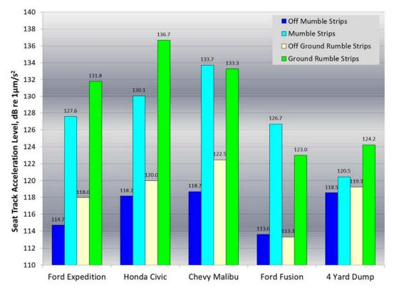
Figure 42: Overall seat track acceleration levels for all five test vehicles on and off mumble strips and ground rumble strips
