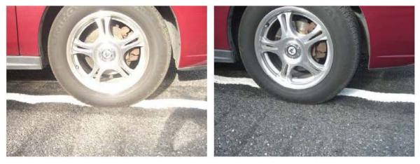
Figure 9: Photographs of the test tire on crest of the mumble strip (left) and in the valley of the mumble strip (right)
