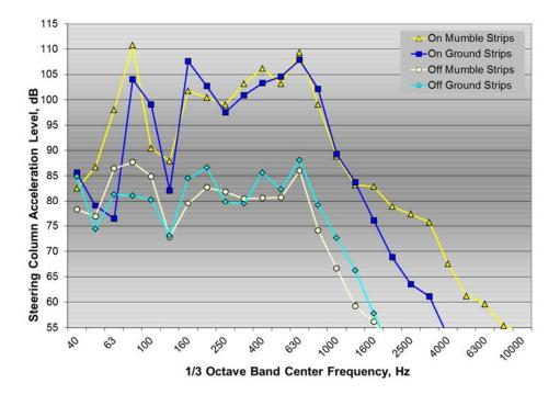
Figure A14:  $\frac{1}{3}$  octave band steering column acceleration spectra for Malibu test vehicle on and off mumble strips and ground rumble strips at 60 mph
