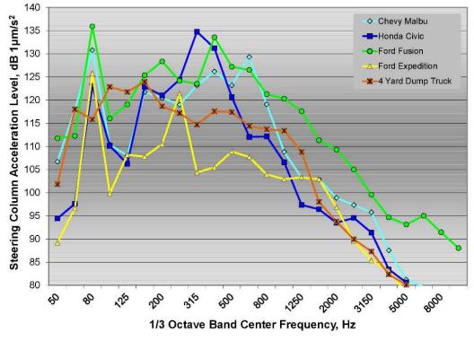
Figure 46:  $\frac{1}{3}$  octave band steering column acceleration spectra for all four test vehicles on mumble strips
