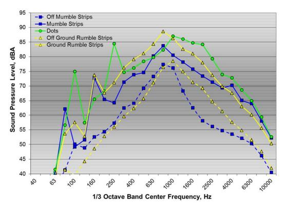
Figure 23:  $\frac{1}{3}$  octave band pass-by spectra for Malibu test vehicle on (solid lines) and off (dashed lines) mumble strips, dots, and ground rumble strips
