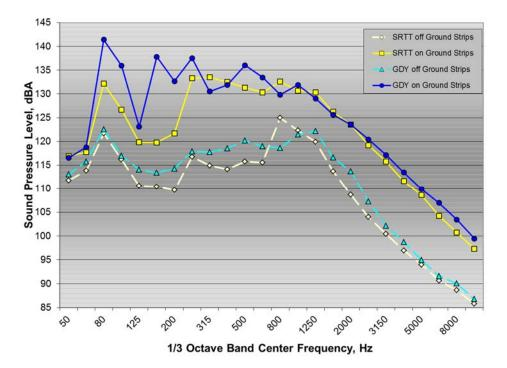
Figure A32:  $\frac{1}{3}$  octave band front fender acceleration spectra for Ford Fusion test vehicle on and off ground rumble strips with SRTT and Goodyear test tires
