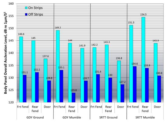
Figure 70: Overall panel acceleration levels on and off warning strips
