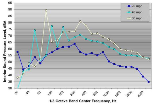
Figure 50:  $\frac{1}{3}$  octave band interior noise spectra on mumble strips for the Malibu test vehicle at 20, 40, and 60 mph
