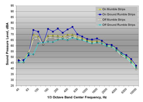
Figure 39:  $\frac{1}{3}$  octave band interior noise spectra for 4-yard dump truck test vehicle on and off mumble strips and ground rumble strips
