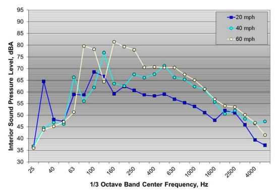
Figure 52:  $\frac{1}{3}$  octave band interior noise spectra on ground rumble strips for the Malibu test vehicle at 20, 40, and 60 mph
