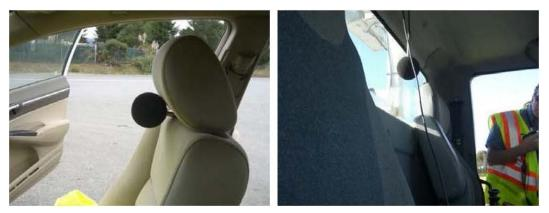
Figure 15: Photographs of the interior noise microphone mounted in the Malibu test vehicle and in the 4-yard dump truck
