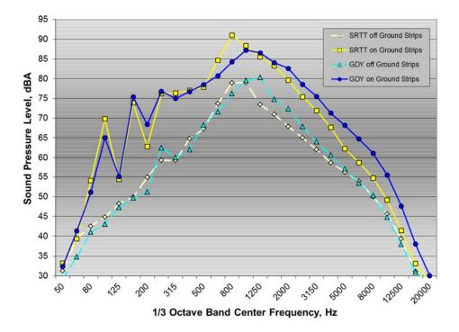
Figure A22: 1/3 octave band pass-by noise spectra for Ford Fusion test vehicle on and off ground rumble strips with SRTT and Goodyear test tires
