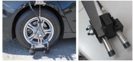
Figure 67: Modified OBSI fixture for rumble strip and mumble strip measurements installed (left) and with added probe holder isolation (right)
