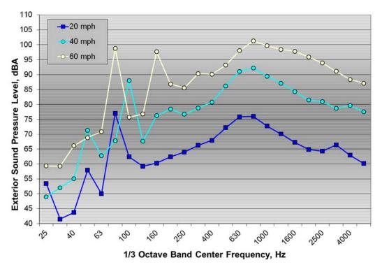
Figure 49:  $\frac{1}{3}$  octave band on-board exterior noise spectra on mumble strips for the Malibu test vehicle at 20, 40, and 60 mph
