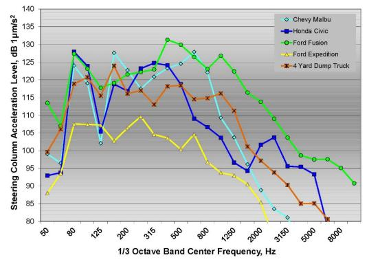
Figure 47:  $\frac{1}{3}$  octave band steering column acceleration spectra for all five test vehicles on ground rumble strips
