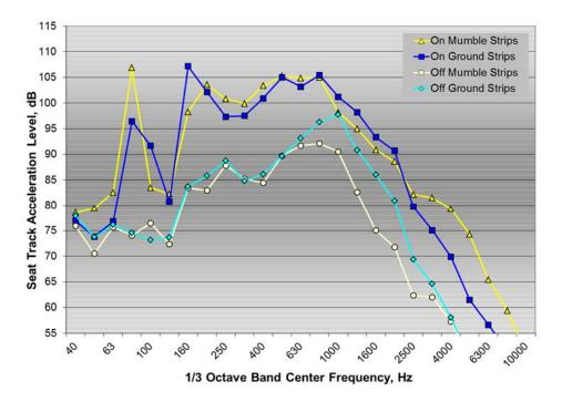
Figure A13:  $\frac{1}{3}$  octave band seat track acceleration spectra for Malibu test vehicle on and off mumble strips and ground rumble strips at 60 mph
