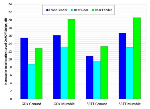
Figure 71: Overall panel acceleration differences for on and off the ground rumble strips and the mumble strips
