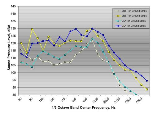
Figure A36:  $\frac{1}{3}$  octave band rear door acceleration spectra for Ford Fusion test vehicle on and off ground rumble strips with SRTT and Goodyear test tires
