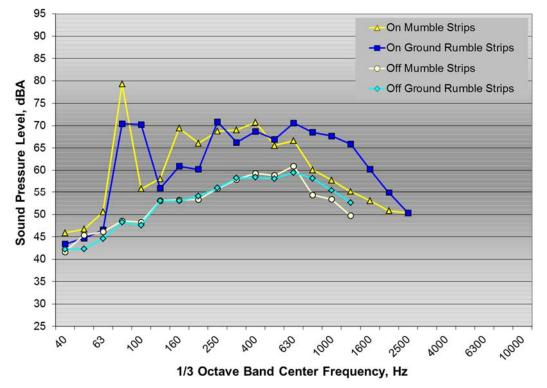
Figure 38:  $\frac{1}{3}$  octave band interior noise spectra for Expedition test vehicle on and off mumble strips and ground rumble strips
