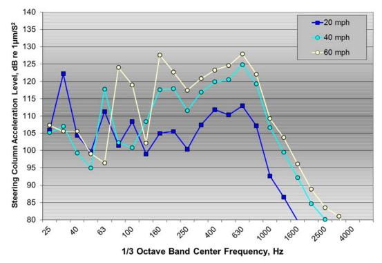
Figure 57:  $\frac{1}{3}$  octave band steering column acceleration level on ground rumble strips for the Malibu test vehicle at 20, 40, and 60 mph
