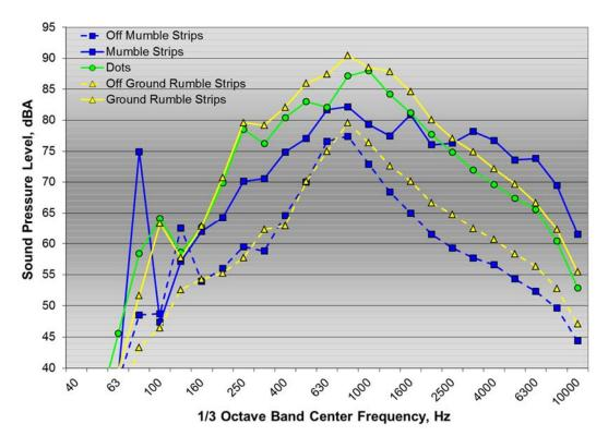
Figure 26:  $\frac{1}{3}$  octave band pass-by spectra for Expedition test vehicle on (solid lines) and off (dashed lines) mumble strips, dots, and ground rumble strips
