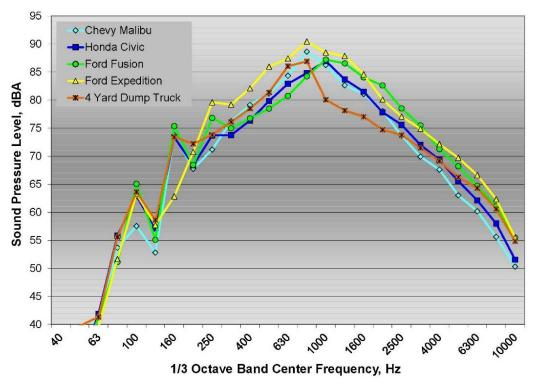
Figure 29: <sup>1</sup>/<sub>3</sub> octave band pass-by spectra on ground rumble strips for all five test vehicles
