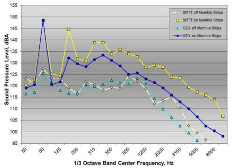
Figure A31:  $\frac{1}{3}$  octave band front fender acceleration spectra for Ford Fusion test vehicle on and off mumble strips with SRTT and Goodyear test tires
