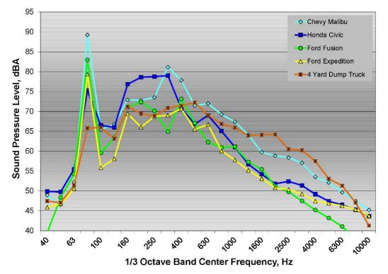
Figure 40: <sup>1</sup>/<sub>3</sub> octave band interior noise spectra for all five test vehicles on mumble strips
