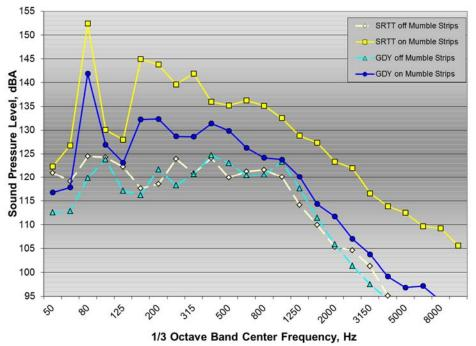
Figure A33:  $\frac{1}{3}$  octave band rear fender acceleration spectra for Ford Fusion test vehicle on and off mumble strips with SRTT and Goodyear test tires
