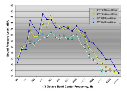
Figure A26:  $\frac{1}{3}$  octave band interior noise spectra for Ford Fusion test vehicle on and off ground rumble strips with SRTT and Goodyear test tires
