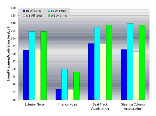
Figure A10: Overall noise and acceleration levels for Malibu test vehicle traveling at 40 mph both on and off ground rumble strips and both eastbound and westbound
