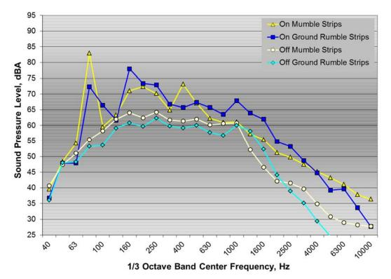
Figure 37:  $\frac{1}{3}$  octave band interior noise spectra for Fusion test vehicle on and off mumble strips and ground rumble strips
