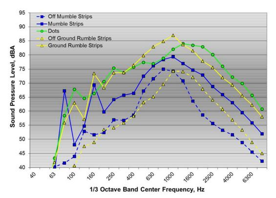
Figure 24:  $\frac{1}{3}$  octave band pass-by spectra for Civic test vehicle on (solid lines) and off (dashed lines) mumble strips, dots, and ground rumble strips
