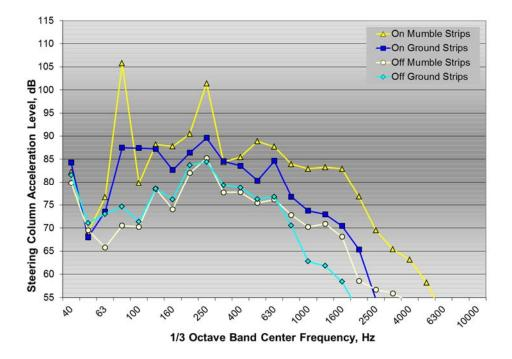
Figure A18: <sup>1</sup>/<sub>3</sub> octave band steering column acceleration spectra for Expedition test vehicle on and off mumble strips and ground rumble strips at 60 mph
