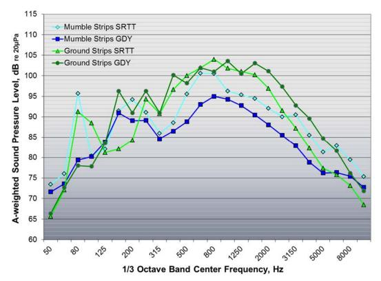
Figure 61: <sup>1</sup>/<sub>3</sub> octave band exterior sound pressure levels measured with GDY tires and SRTT
