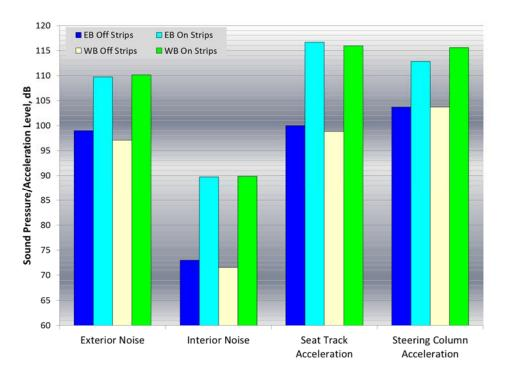
Figure A4: Overall noise and acceleration levels for Civic test vehicle traveling at 60 mph both on and off ground rumble strips and both eastbound and westbound
