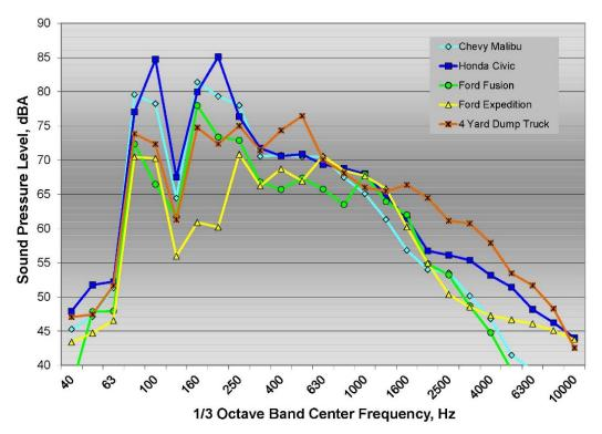
Figure 41: <sup>1</sup>/<sub>3</sub> octave band interior noise spectra for all five test vehicles on ground rumble strips
