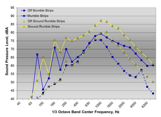
Figure 25:  $\frac{1}{3}$  octave band pass-by spectra for Ford Fusion test vehicle on (solid lines) and off (dashed lines) mumble strips and ground rumble strips
