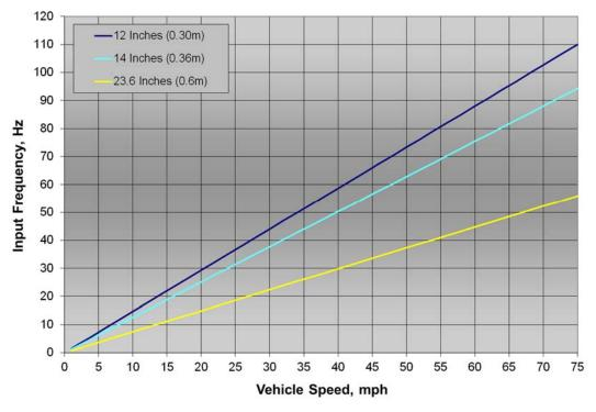
Figure 6: Forcing function frequency as a function of vehicle speed for different  $\lambda$  values
