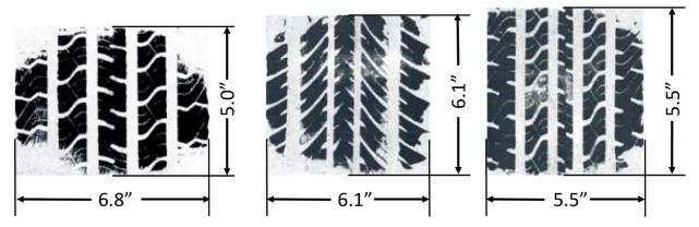
Figure 2: Tire contact patch geometries for three typical size passenger car tires: SRTT reference tire, Goodyear Aquatred III, and Uniroyal Tiger Paw (left to right)
