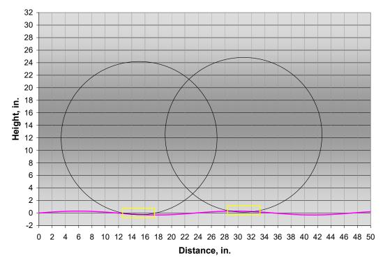
Figure 4: Relative geometries of typical passenger car tire, tire contact patch length, and exaggerated rumble strip profiles of  $\lambda$ =23.6 inches
