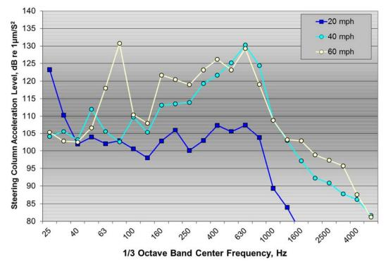
Figure 55:  $\frac{1}{3}$  octave band steering column acceleration level on mumble strips for the Malibu test vehicle at 20, 40, and 60 mph
