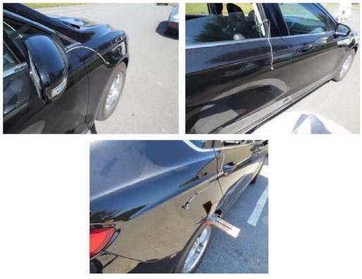
Figure 69: Body panel acceleration measurement points: front fender (upper left), rear door (upper right), and rear fender (lower center)
