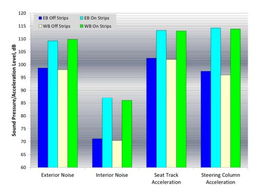
Figure A8: Overall noise and acceleration levels for Malibu test vehicle traveling at 60 mph both on and off ground rumble strips and both eastbound and westbound
