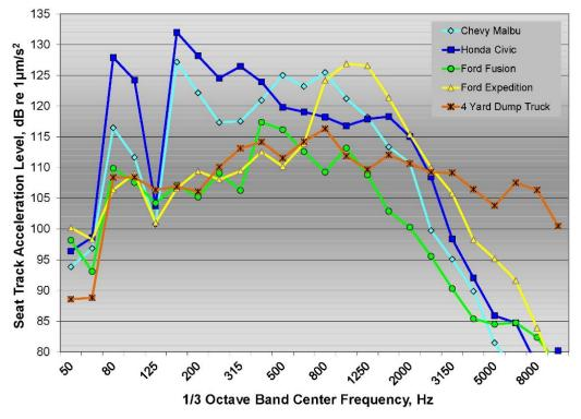
Figure 44:  $\frac{1}{3}$  octave band seat track acceleration spectra for all five test vehicles on ground rumble strips
