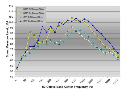
Figure A24: 1/3 octave band exterior noise spectra for Ford Fusion test vehicle on and off ground rumble strips with SRTT and Goodyear test tires
