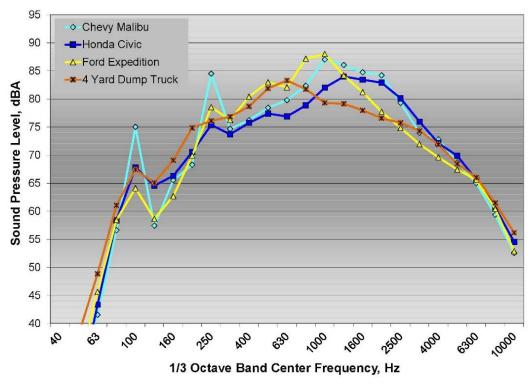
Figure 30: 1/3 octave band pass-by spectra on dots for four test vehicles
