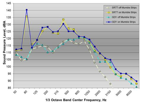
Figure A29:  $\frac{1}{3}$  octave band steering column acceleration spectra for Ford Fusion test vehicle on and off mumble strips with SRTT and Goodyear test tires
