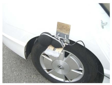
Figure 14: Photograph of on-board microphone mounted above the wheel opening at the right rear tire of the Civic test vehicle
