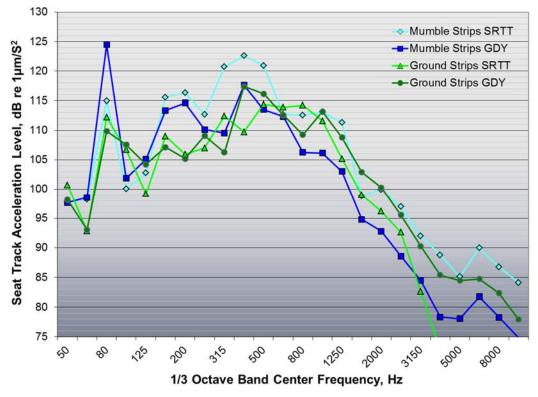
Figure 64: 1/3 octave band seat track acceleration levels measured with GDY tires and SRTT
