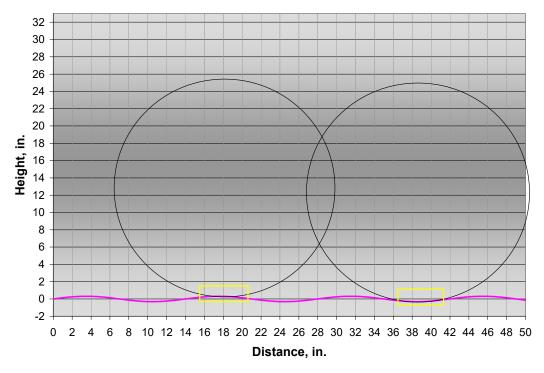
Figure 5: Relative geometries of typical passenger car tire, tire contact patch length, and exaggerated rumble strip profiles  $\lambda$ =14 in.
