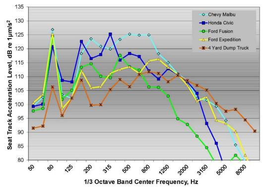
Figure 43:  $\frac{1}{3}$  octave band seat track acceleration spectra for all five test vehicles on mumble strips
