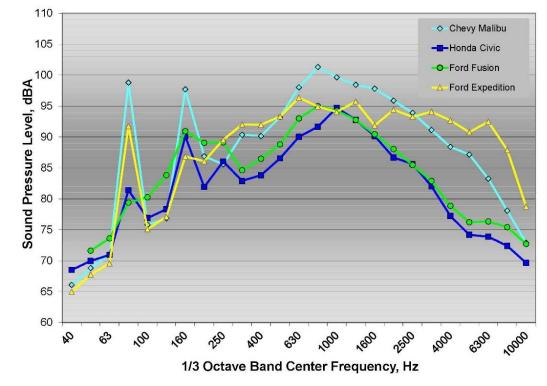
Figure 32: <sup>1</sup>/<sub>3</sub> octave band on-board exterior spectra on mumble strips for four test vehicles
