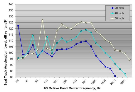
Figure 54:  $\frac{1}{3}$  octave band seat track acceleration level on mumble strips for the Malibu test vehicle at 20, 40, and 60 mph
