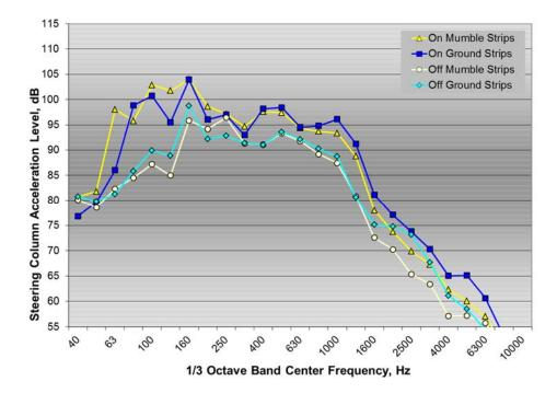
Figure A20:  $\frac{1}{3}$  octave band steering column acceleration spectra for 4-yard dump truck test vehicle on and off mumble strips and ground rumble strips at 60 mph
