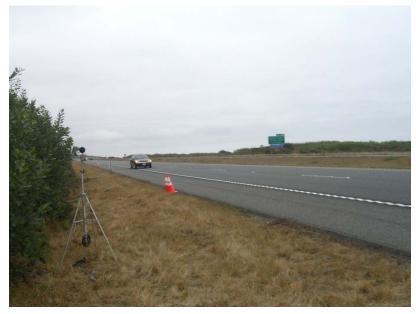
Figure 13: Photograph of Malibu pass-by measurement on the mumble strips on US Highway 101
