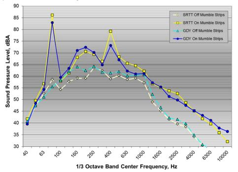
Figure A25:  $\frac{1}{3}$  octave band interior noise spectra for Ford Fusion test vehicle on and off mumble strips with SRTT and Goodyear test tires
