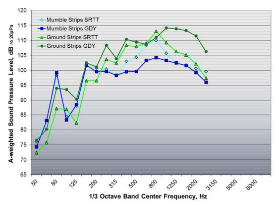
Figure 68:  $\ensuremath{^{1}\!\!\!\!\!\!\!\!\!\!\!\!\!}_3$  octave band sound pressure levels measured by the OBSI probes for the GDY tires and SRTT
