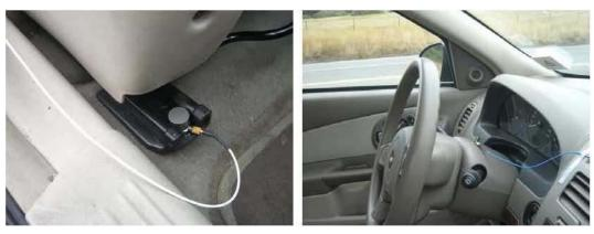
Figure 16: Photographs of accelerometers mounted on the seat track (left) and the steering column (right) on the Malibu test vehicle
