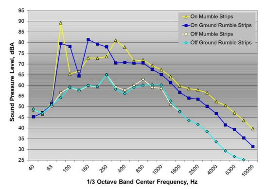
Figure 35:  $\frac{1}{3}$  octave band interior noise spectra for Malibu test vehicle on and off mumble strips and ground rumble strips
