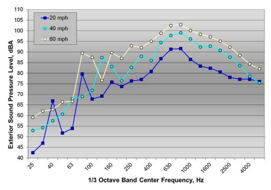
Figure 51:  $\frac{1}{3}$  octave band on-board exterior noise spectra on ground rumble strips for the Malibu test vehicle at 20, 40, and 60 mph
