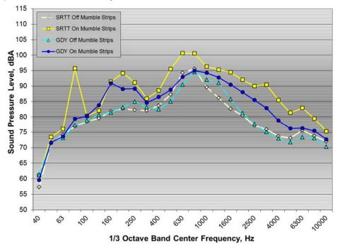
Figure A23:  $\frac{1}{3}$  octave band exterior noise spectra for Ford Fusion test vehicle on and off mumble strips with SRTT and Goodyear test tires
