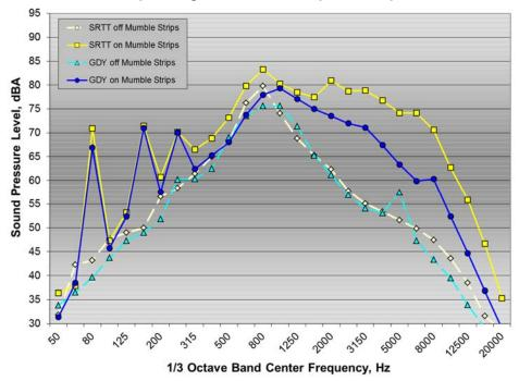
Figure A21:  $\frac{1}{3}$  octave band pass-by noise spectra for Ford Fusion test vehicle on and off mumble strips with SRTT and Goodyear test tires
