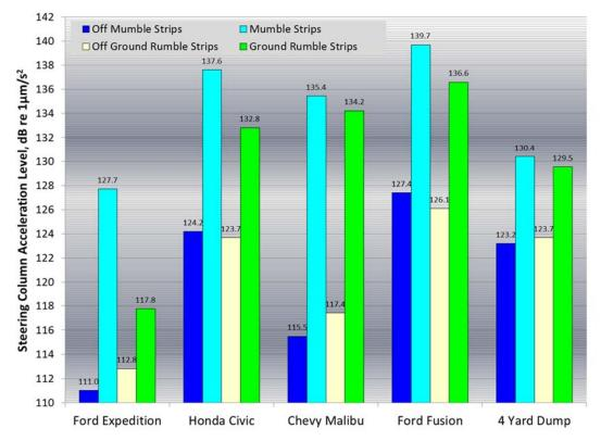
Figure 45: Overall steering column acceleration levels for all five test vehicles on and off mumble strips and ground rumble strips
