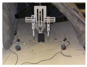
Figure 18: In-lab testing to detect reflections or other effects of CPX 2 probe SI fixture on sound pressure levels received at the CPX microphone locations using a loudspeaker source in July 2003 (measurements made with the ADOT trailer door closed)
