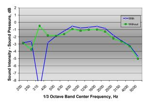
Figure 14: Comparison of 1/3 octave band differences bewteen SI and SPL levels with and without nose cones for a windscreen protected probe measured on PCC pavements on the Mojave Bypass
