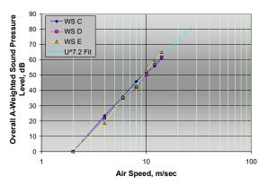
Figure 6a: Microphone windscreen performance for normally incident flow spanning range of production variation for commercially available windscreens
