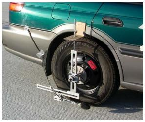
Figure 3: Configuration for SI application to tire/pavement noise measurement for purposes of quantifying highway pavement performance as employed on Caltrans projects starting in 2002
