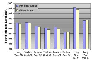
Figure 12: Comparison of overall SI levels with and without nose cones for a windscreen protected probe measured on PCC pavements on the Mojave Bypass
