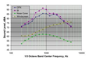
Figure 9: Comparison of flow induced noise (SPL) for a nose cone and a windscreen protected microphone relative to CPX & SI tire noise
