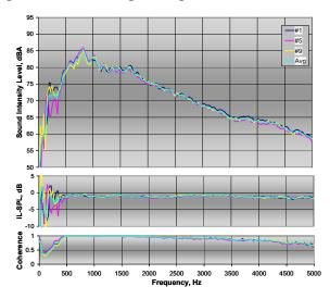
Figure 29: SI for multiple runs on ARFC for the leading edge of the tire contact patch using the dual probe fixture
