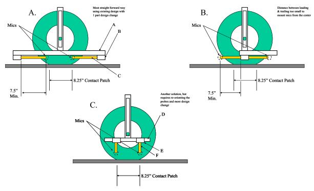
Figure 17: Alternative configurations conceptualized for a two probe tire/pavement noise SI measurement method
