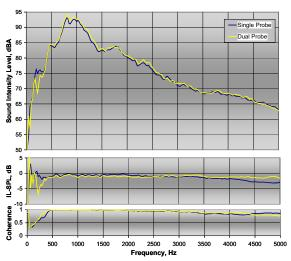
Figure 34: Comparison single and dual probe SI averages of multiple runs on grind #2 PCC for the leading edge of the tire contact patch
