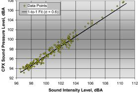
Figure 20: SI vs. CPX tire/pavement noise levels measured simultaneously on the ADOT CPX trailer using a two probe SI fixture
