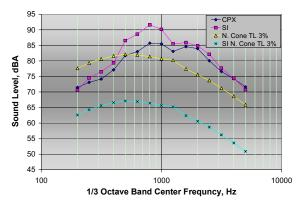
Figure 11: Comparison of the flow induced background noise for SPL and IL using nose cones with a 3% turbulence level relative CPX & SI tire/payement noise
