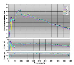
Figure 31: SI for multiple runs on ARFC for the trailing edge of the tire contact patch using the single probe fixture
