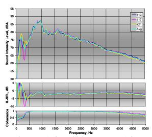
Figure 32: SI for multiple runs on ARFC for the trailing edge of the tire contact patch using the dual probe fixture
