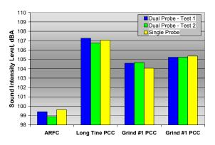
Figure 23: Comparison of overall Aweighted SI levels measured with single and dual probe fixtures on 4 pavements
