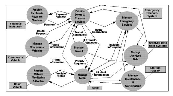
Figure 12-2 Example of Logical Architecture
