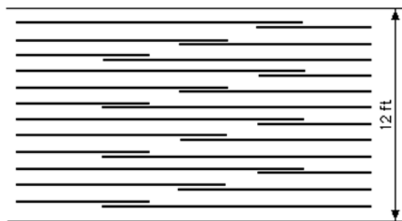
Figure 200–2: Staggered lap splices
