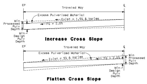
Figure 9. Slope Corrections and Minimum Design Pulverization Depth
