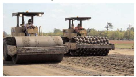
Figure 3. Steel Drum Roller and Sheepsfoot Roller (no blade)
