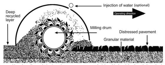
Note: depending on the in-situ moisture content, water may be injected in the mixing drum during pulverization.
