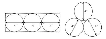
Figure 6c. Examples of Clustered Coring Patterns
