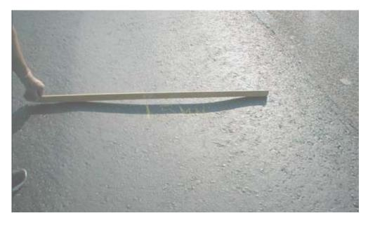
Figure 5. Pavement Surface Rutting (over ¾ inch) Suitable for Pulverization.
