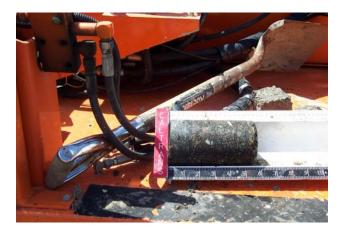
Figure 6b. Core (4 Inch Diameter)
