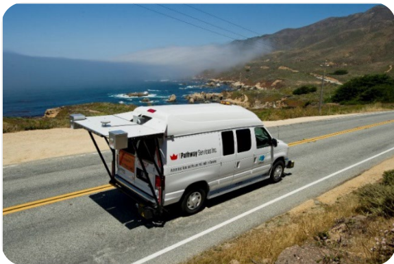
FIGURE 1. A.P.C.S. VEHICLE ON THE ROAD AND MANUAL PAVEMENT INSPECTION
