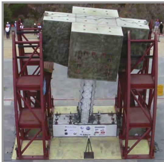
*Beaten, but not broken, a full-scale Caltrans-designed bridge column on the UCSD/NEES Outdoor Shake Table maintains vertical support of more than 260 tons after undergoing six simulated earthquakes, each in excess of maximum design load.*
