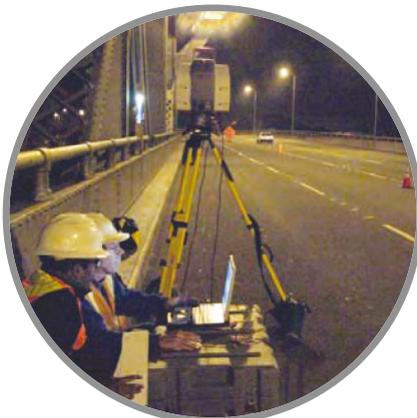
*Night scanning of the old Bay Bridge for the design and construction of the new Bay Bridge detour in District 4*
