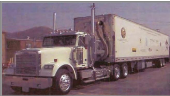
The UC Riverside mobile emissions laboratory (MEL) is a unique laboratory containing all the instrumentation normally found in a conventional vehicle emissions laboratory but mounted inside a 53-foot truck trailer.
