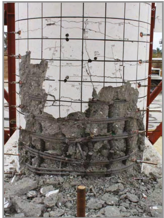
*Close-up view of ductile fuse at column base after completion of all testing*
