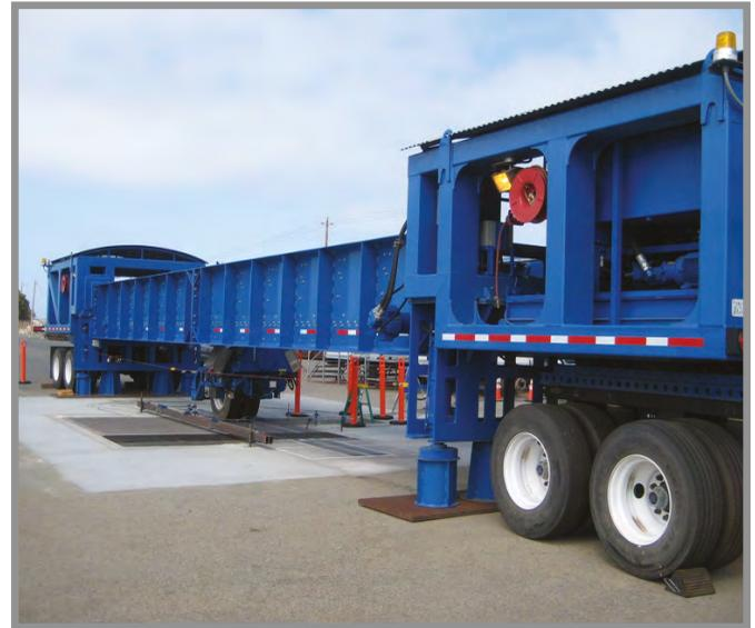
*HVS testing on the deck joint*
