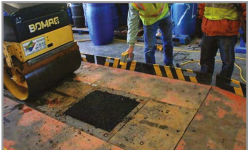
HMA materials being compacted in the laboratory for testing
