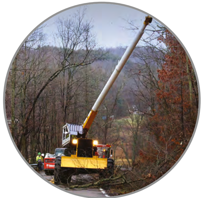
Jarraff all-terrain rotary tree trimmer lets the operator remain in an enclosed cab safely away from cutting blades and falling debris.
