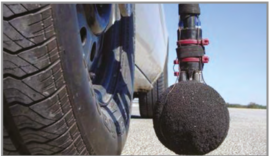
Measuring tire pavement noise
