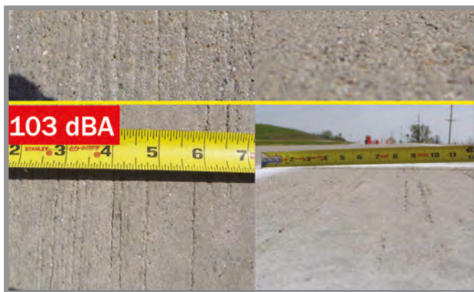
Variability of drag texture surface and its effect on overall OBSI level
