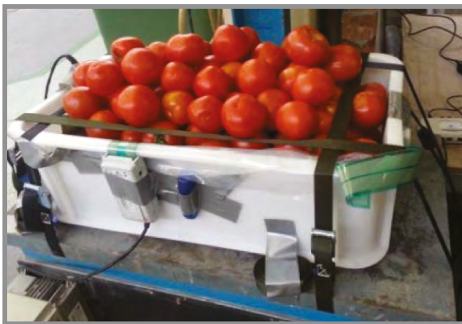
Laboratory testing of damage to tomatoes from imposed vibrations
