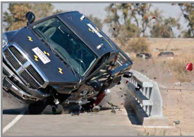
Vehicle impacting the barrier
