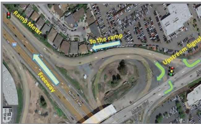
Outer diagonal ramp with two feeding movements
