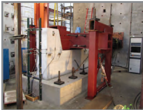
Test of a non-skewed shear key (left) and skewed shear key (right)
