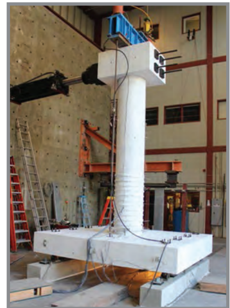
Specimen 1 used a 9.8 bar diameter embedment length for the headed bars.
