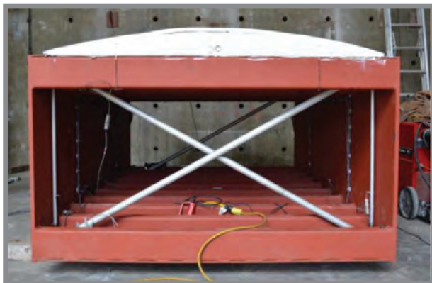
One-ninth scale steel tunnel to assess the interaction between the tunnel liner and the surrounding ground
