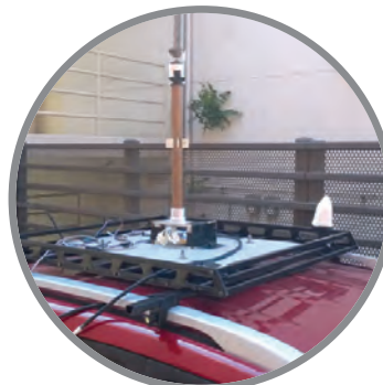
Receiver array on top of the vehicle
