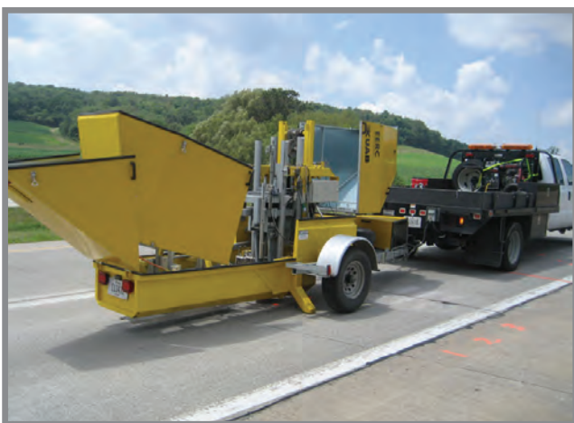
Evaluating the physical properties of concrete pavement over a polyurethane foam-stabilized base using a falling weight deflectometer device
