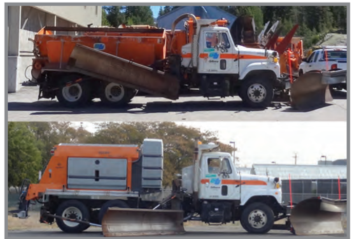
Profile of the Kingvale plow truck with V-box (above) and Epoke (below) spreaders installed
