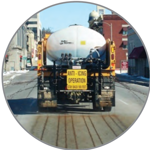
Stripes of liquid behind a low-tech brining truck
