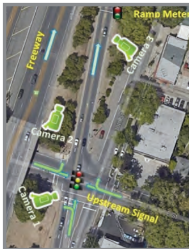
Typical camera layout for queue storage data collection
