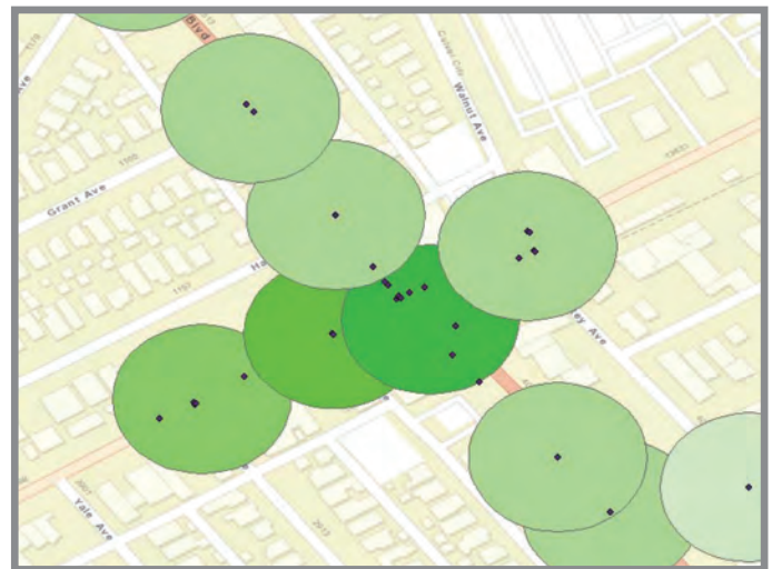
Crashes clustered using 50-foot buffers. The darker the green, the higher the number of crashes. The intersection was identified as a high-crash location.
