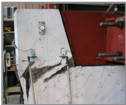
Failure behavior of a non-isolated shear key
