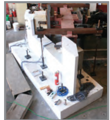
Test of a non-skewed shear key (left) and skewed shear key (right)
