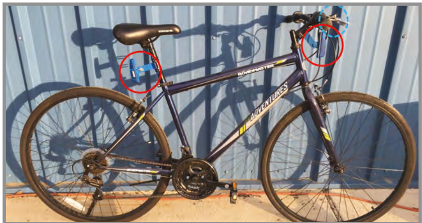
Commuter bicycle instrumented with accelerometers (red circles) at the typical mounting locations and a GPS unit on the handlebar (blue dashes).
