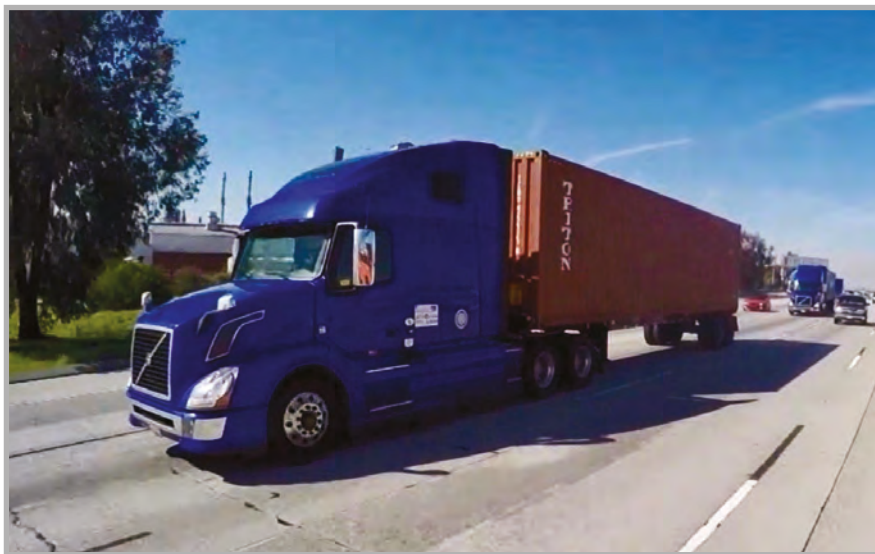
Electronically coupled Volvo trucks modified by UC Berkeley PATH showing truck platooning operations at a 2017 Caltrans demonstration on the I-110 near the Port of Los Angeles
