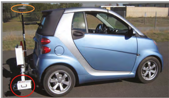
Lightweight inertial profiler with rear-mounted high-speed lasers, one in each wheel path (red circle) and GPS unit (orange circle).
