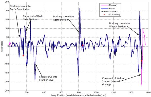
Figure 5-38 EmX EB run: steering angle and command of the steering wheel (distance based)
