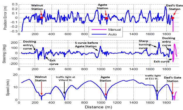
Figure 5-39 EmX WB revenue service run: lateral position error, steering wheel angle, and speed (distance based)
