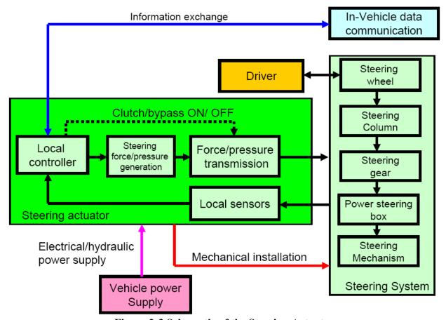
Figure 2-3 Schematic of the Steering Actuator
