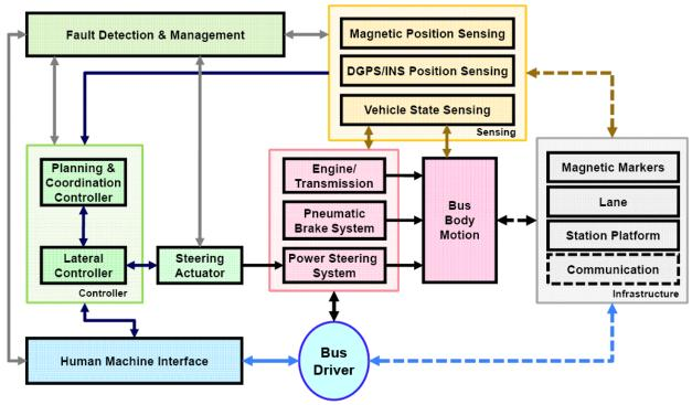
Figure 1-1 Functional Block Diagram of the VAA System
