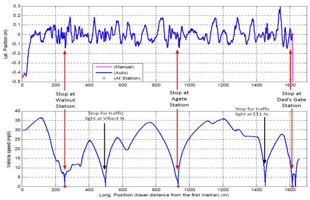
Figure 5-32 EmX WB run: lateral position error and speed (distance based)
