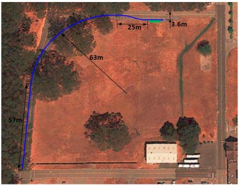
Figure 5-4 The test track at Richmond Field Station (Map View)
