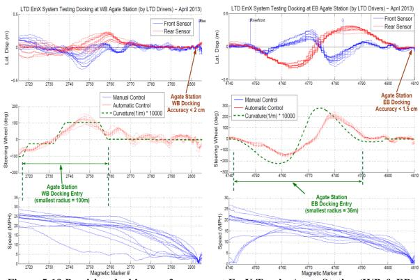
Figure 5-19 Precision docking performance at EmX Track: Agate Station (WB & EB)
