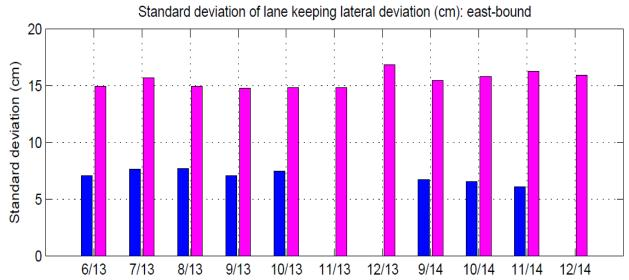
Figure 5-45 Standard deviation of lane keeping deviation for each month of revenue service (blue: automated steering, magenta: manual steering)
