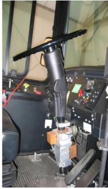
Figure 3-4 New Flyer steering wheel and column (60' Diesel)
