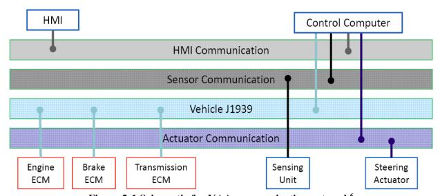
Figure 2-1 Schematic for VAA communication network<sup>6</sup>
