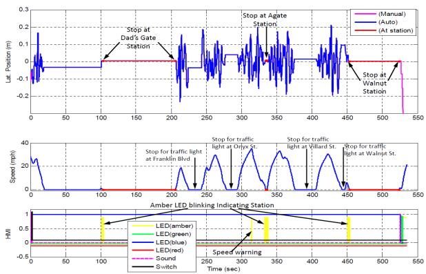
Figure 5-35 EmX EB run: lateral position error, speed, and HMI LEDs & switch (time based)
