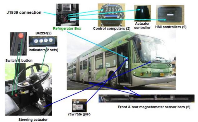
Figure 3-8 VAA system components and installation on the LTD 60-ft New Flyer bus
