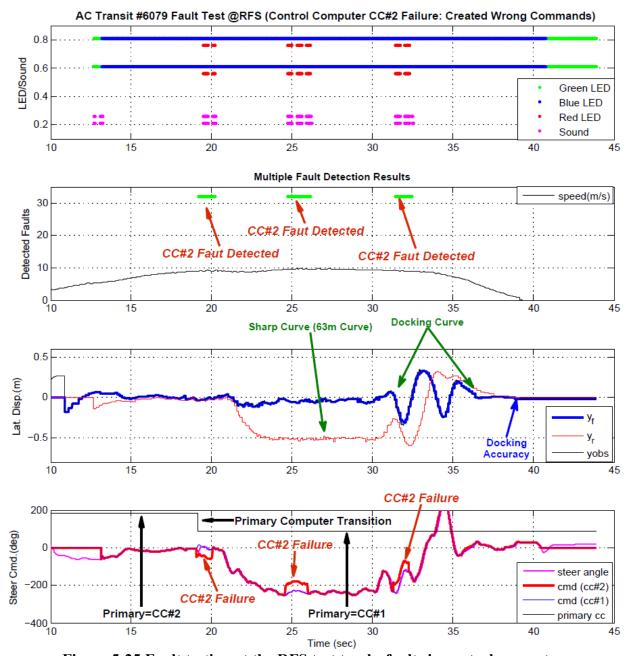
Figure 5-25 Fault testing at the RFS test track: faults in control computers
