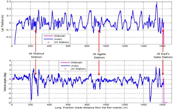
Figure 5-33 EmX WB run: lateral position error and vehicle angle (distance based)
