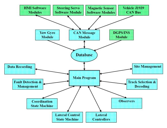
Figure 3-7 VAA System Software Architecture
