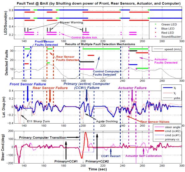
Figure 5-21 Fault testing on EmX conducted by the LTD instructors
