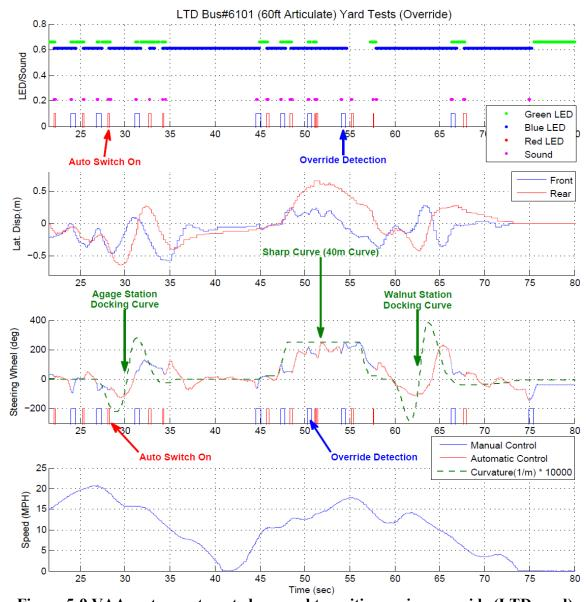
Figure 5-9 VAA system automated-manual transitions using override (LTD yard)
