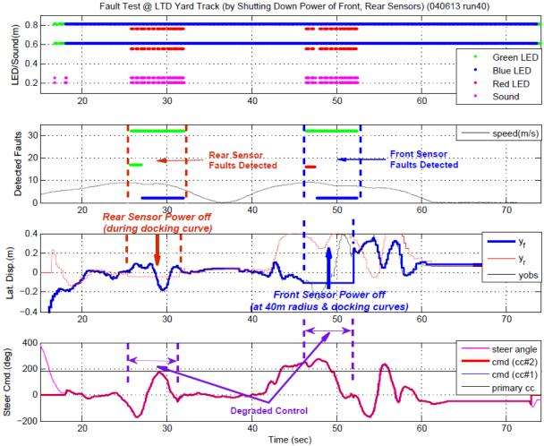
Figure 5-10 Fault testing at the LTD yard track: fault in the rear and front sensors (degraded control set to continuously sustain the automated functions)
