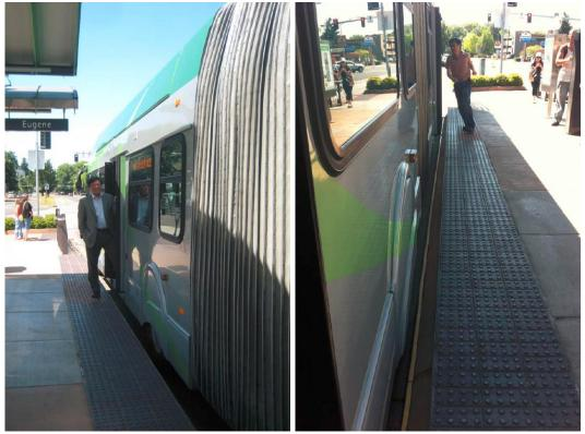
Figure 5-27 Precision docking at Agate Station (west-bound and east-bound)
