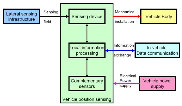
Figure 2-2 Schematic for Vehicle Position Sensing
