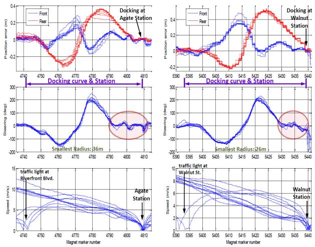
Figure 5-42 Docking performance at EB Agate Station (left) and EB Walnut Station (right) (One day's of revenue service data)
