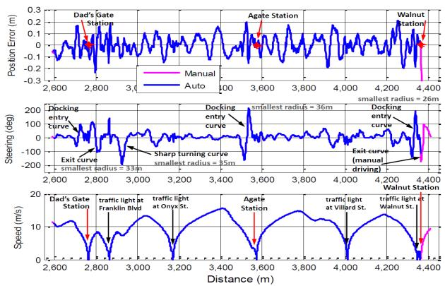
Figure 5-40 EmX EB revenue service run: lateral position error, steering wheel angle, and speed (distance based)
