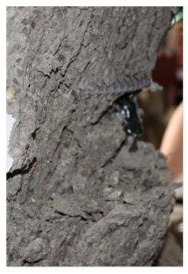
Figure 3.8 - Buckled bar #1 at south face of Specimen #1 during  $2^{nd}$  cycle of -8% drift
