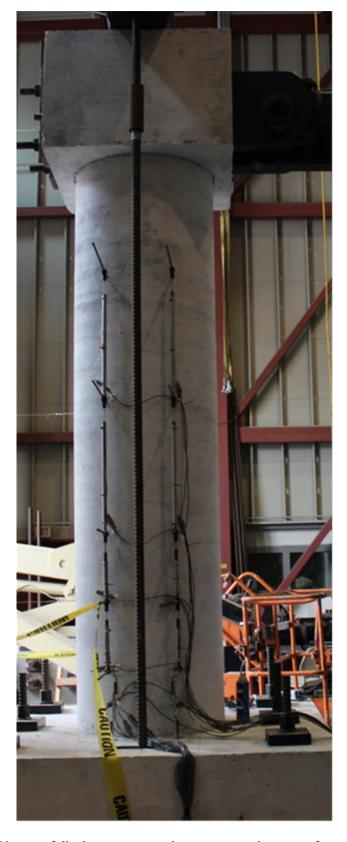
Figure 2.13 - Picture of displacement transducers mounted on west face of Specimen #1
