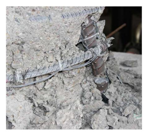
Figure 3.11 – Fractured bar #4 at north face of Specimen #1 during 2<sup>nd</sup> cycle of -10% drift
