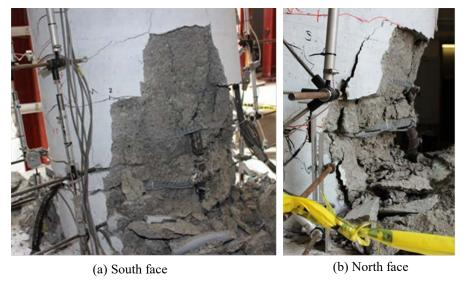
Figure 3.10 - Crushing in Specimen #1 during  $2^{nd}$  cycle of +10% drift
