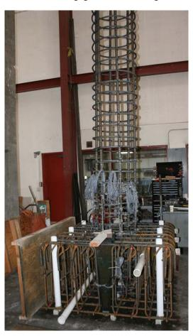
Figure 2.18 - Reinforcement cage for Specimen #1
