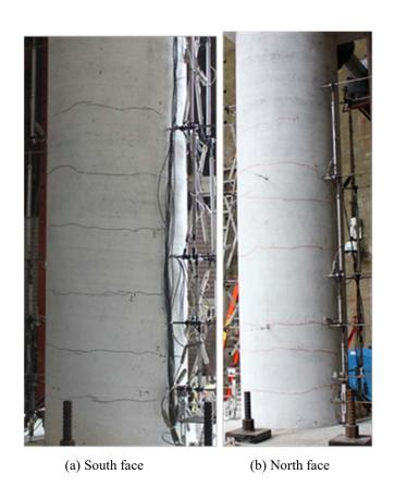
Figure 3.4 – Specimen #1 at 1% drift
