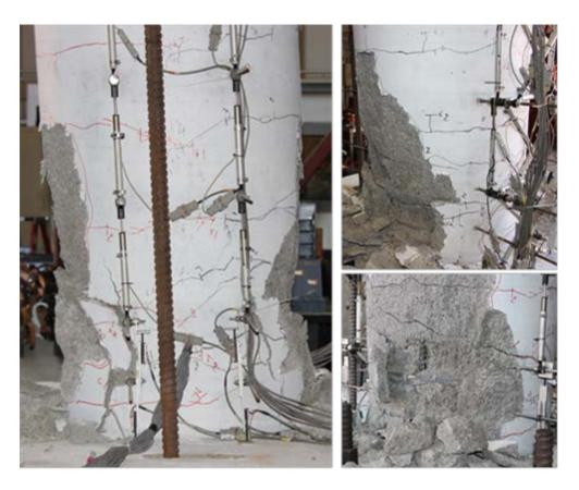
Figure 3.20 - Specimen #2 at 6% drift
