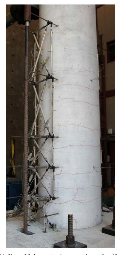
Figure 2.14 – Picture of displacement transducers mounted on east face of Specimen #2
