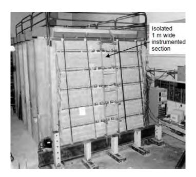
Figure 3.1. Full-scale GRS retaining wall facility at RMC (Bathurst et al. 2000).
