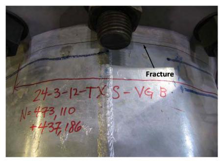
Figure 5.2: Base Plate Weld Fracture
