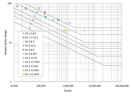
Figure 6.13: Experimental Fatigue Life vs. Hot spot Stress
