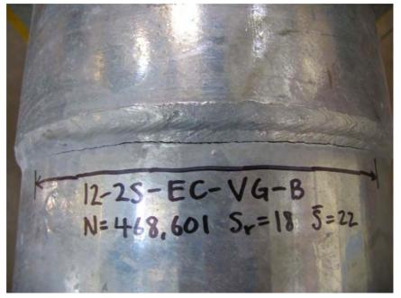
Figure 3.7: Typical External Collar Failure
