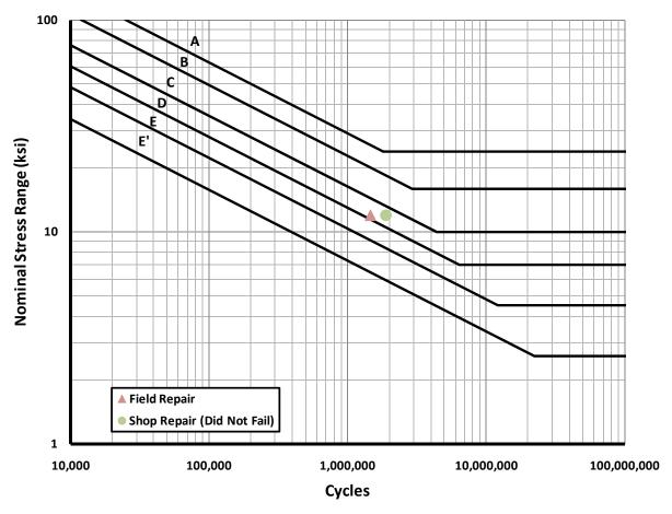
Figure 7.22: S-N Plot of Weld Repair Specimens
