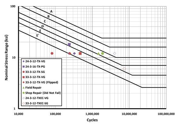
Figure 7.27: S-N Plot of All Specimens
