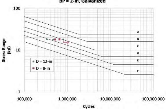
External Collar Pole Diameter BP = 2-in, Galvanized
