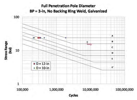
Figure 3.16: Comparison of Mast Arm Diameter, 3-in. Base Plate Full Penetration Details
