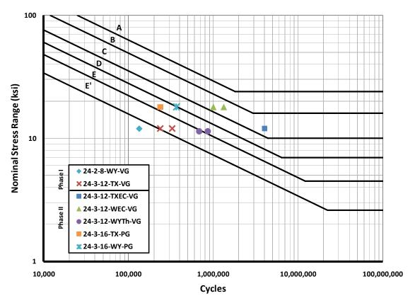
Figure 5.12: Full Penetration Results for Phases I and II
