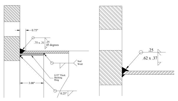
Figure 1.3: Full Penetration Weld Detail—Texas on Right, Wyoming on Left
