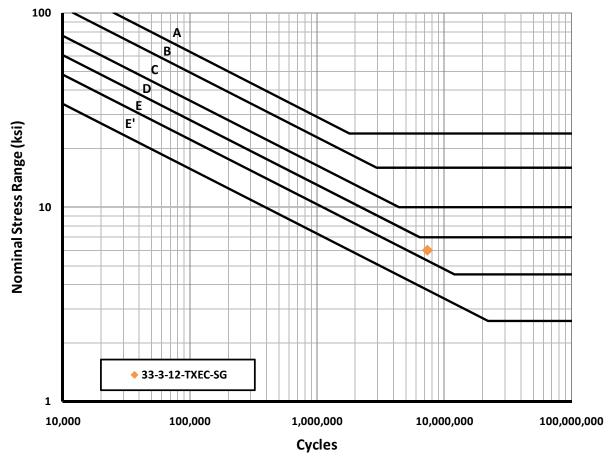
Figure 7.25: S-N Plot of External Collar Samples
