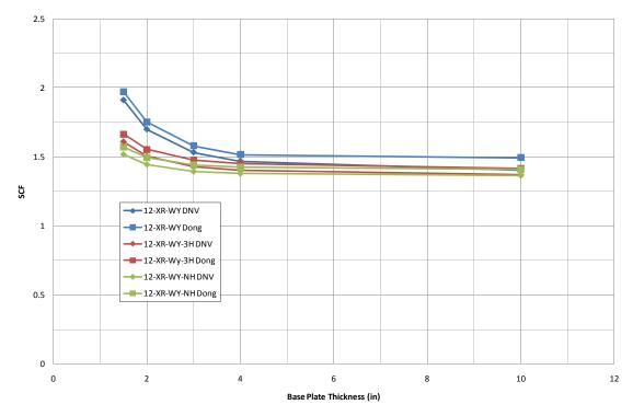
Figure 4.13: Base Plate Hole Evaluation (SCF versus Base Plate Thickness)
