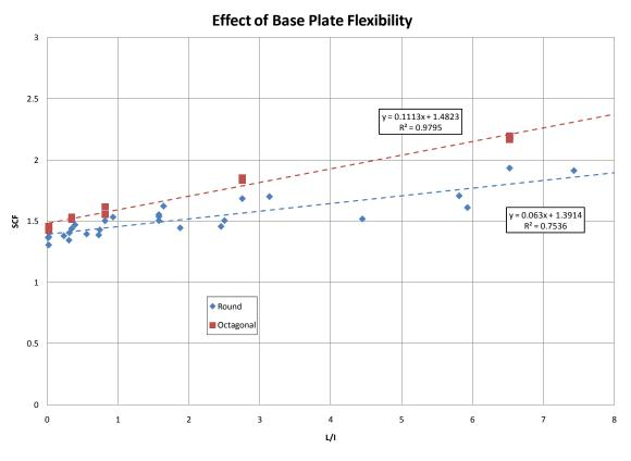
Figure 4.16: SCF versus Base Plate Flexibility (Constant Applied Moment)
