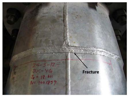
Figure 5.3: Collar Weld Fracture
