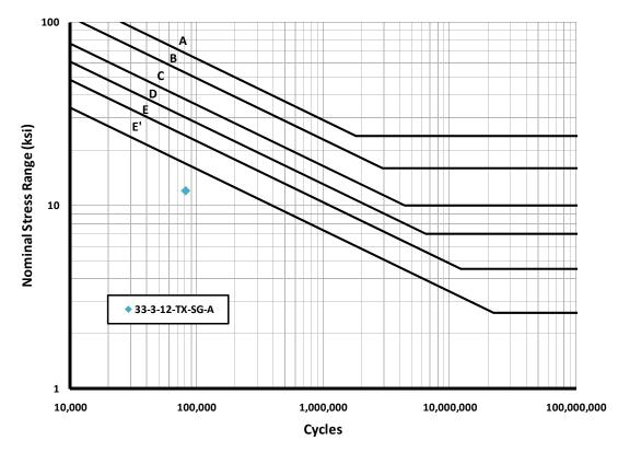
Figure 7.5: Fatigue Life of Galvanized Specimen Compared to AASHTO Fatigue Categories
