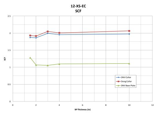
Figure 4.19: 12-XS-EC (SCF versus Base Plate Thickness)
