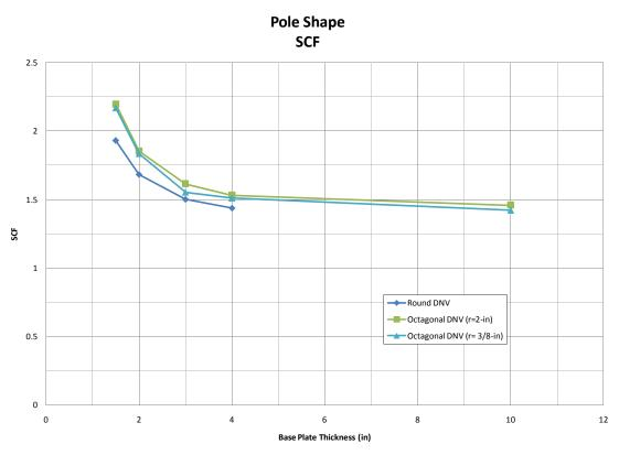
Figure 4.9: Mast arm Shape Evaluation (SCF versus Base Plate Thickness)
