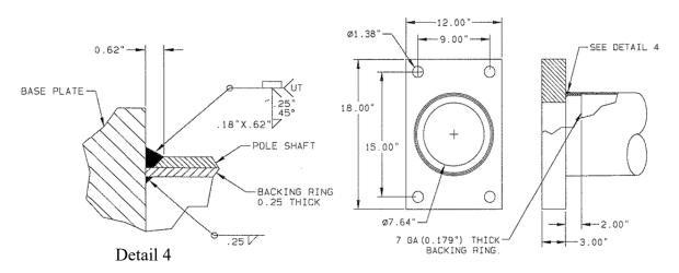
Figure 8.2: Full Penetration Weld Detail
