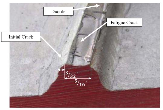
Figure 7.8: Depth of Initial Crack at Weld Toe
