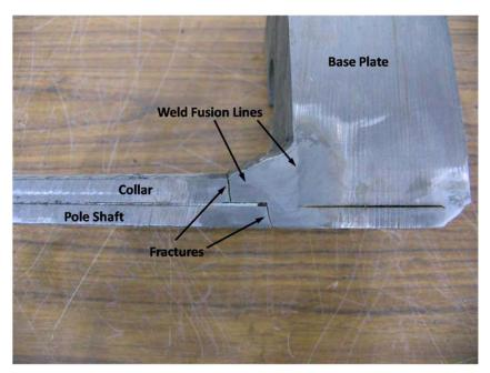
Figure 5.5: Section of Valmont Socket External Collar Connection
