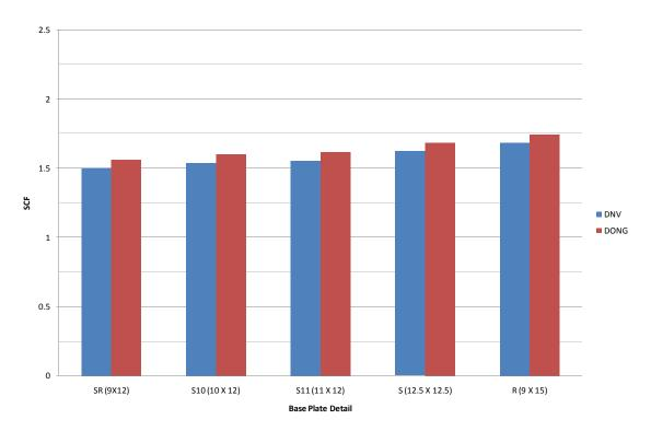
Figure 4.12: Base Plate Geometry Evaluation (SCF)
