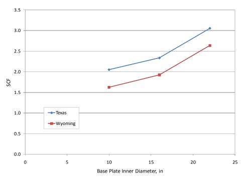
Figure 6.8: Results of Base Plate Inner Diameter Parametric Evaluation
