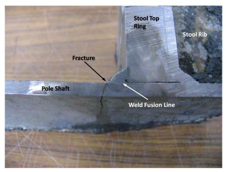
Figure 5.8: Section of Stool Detail Fillet Weld
