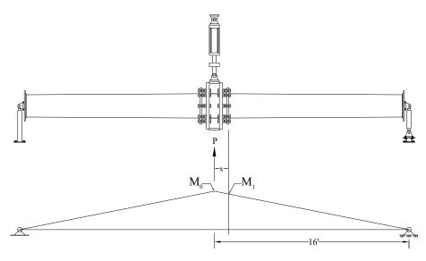
Figure 2.7: Moment Diagram for Calculating Testing Loads (Rios, 2007)
