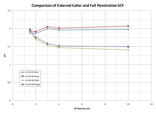
Figure 4.20: Comparison of External Collar and Full Penetration SCF
