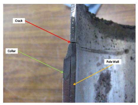
Figure 3.9: Close-up of the Collar Weld (Etched)
