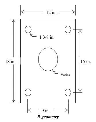
Figure 1.4: Square and Rectangular Mast Arm Base Plates
