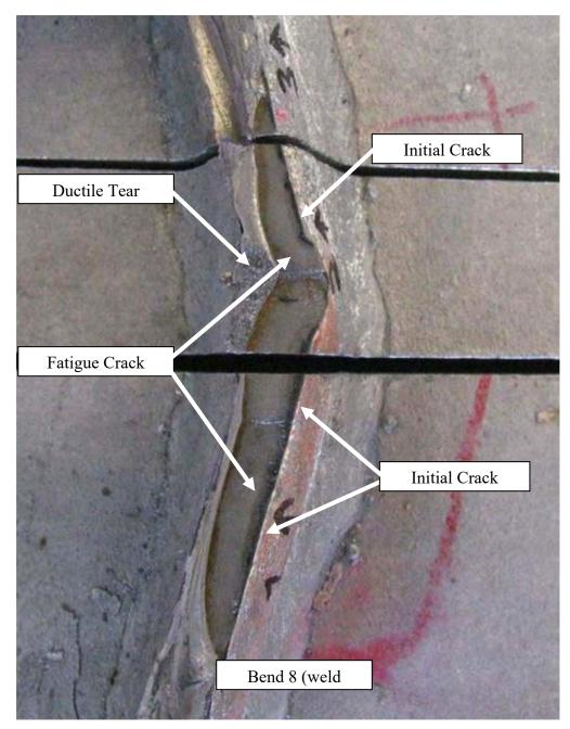
Figure 7.11: Fracture Surface of Bend 8
