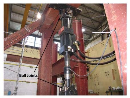
Figure 2.4: MTS 55-kip Hydraulic Actuator
