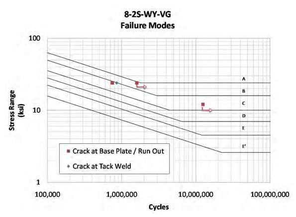
Figure 3.19: Variation of Backing Ring Welds, 8-2S-WY
