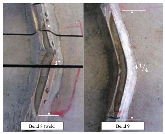
Figure 7.10: Fatigue Cracks at Bends 8 and 9
