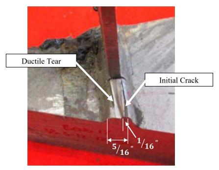
Figure 7.9: Fracture Surface at Bend 12
