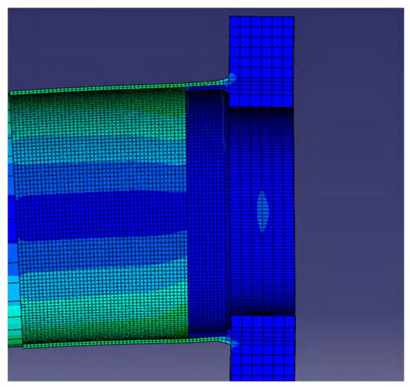
Figure 4.5: Bending in the Base Plate Connection (12-3R-WY)
