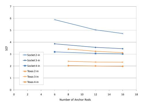
Figure 6.6: Results of Anchor Rod Parametric Evaluation
