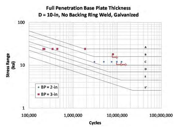
Figure 3.14: Comparison of 2-in. and 3-in. Full Penetration Details
