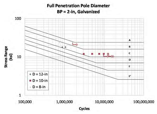
Figure 3.15: Comparison of Mast arm Diameter, 2-in. Base Plate Full Penetration Details
