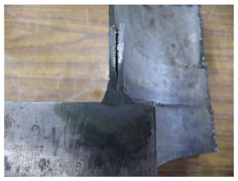
Figure 3.2: Cross Section of a Typical Full Penetration Connection
