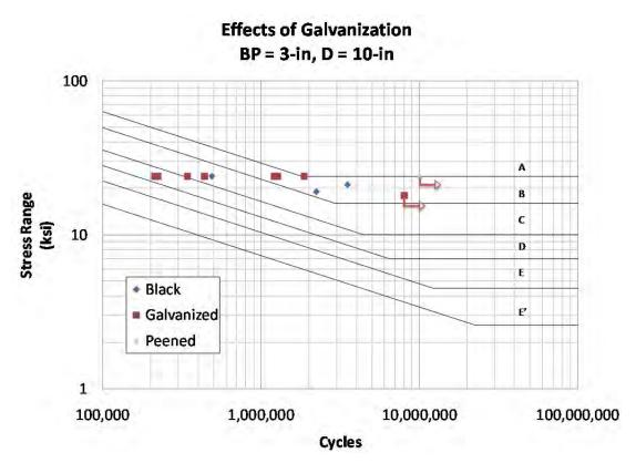
Figure 3.21: Comparison of Galvanized, Black, and Peened 10-3R-WY
