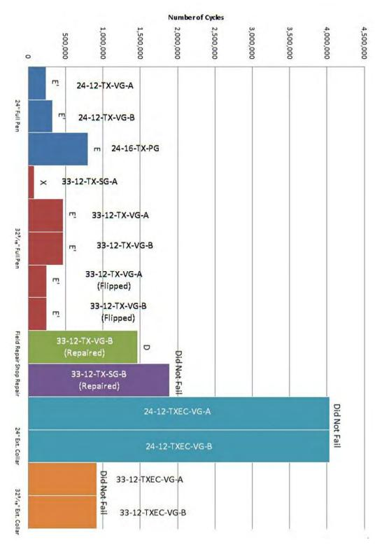
Figure 7.28: Fatigue Results by Specimen Normalized for 12-ksi Stress Range
