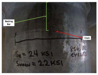
Figure 3.5: Typical Failure at a Backing Ring Tack Weld
