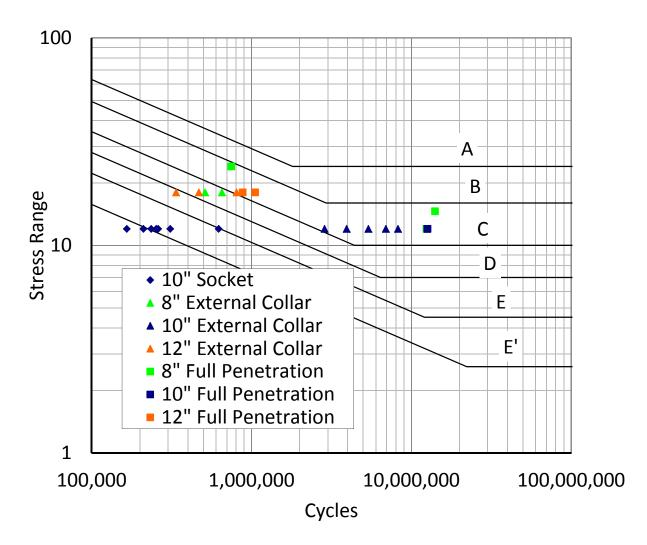
Figure 8.1: Mast Arm Fatigue Test Results—2-in. End Plates
