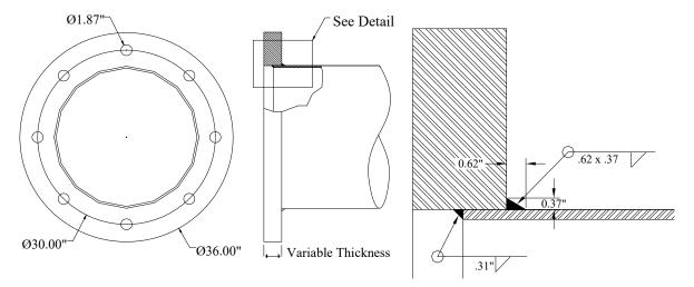
Figure 1.1: Socket Connection
