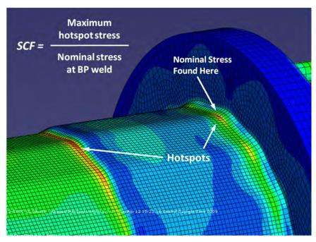
Figure 6.1: Analytical Model with Multiple Hot Spot Locations
