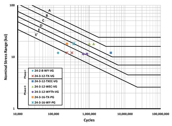
Figure 8.4: Fatigue Performance of High-mast Details
