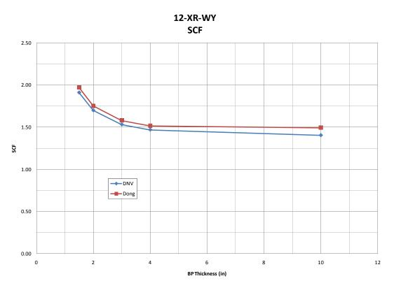
Figure 4.3: 12-XR-WY (SCF versus Base Plate Thickness)
