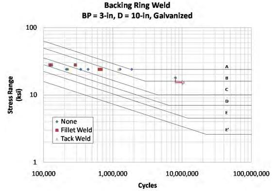
Figure 3.18: Variation of Backing Ring Weld, 10-3R-WY
