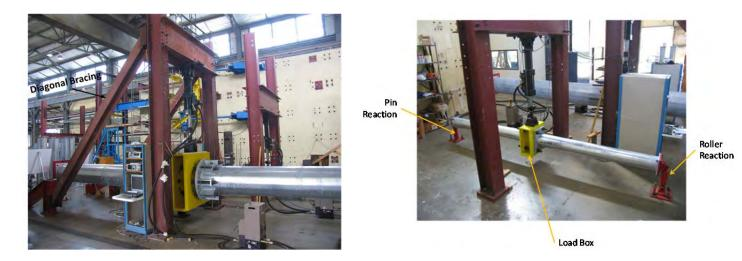
Figure 2.3: Portal Loading Frame High-mast and Mast Arm Tests
