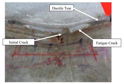
Figure 7.17: Bend 3 of Specimen 33-3-12-TX-VG-A
