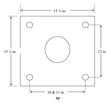
Figure 4.11: Intermediate Base Plate Geometry
