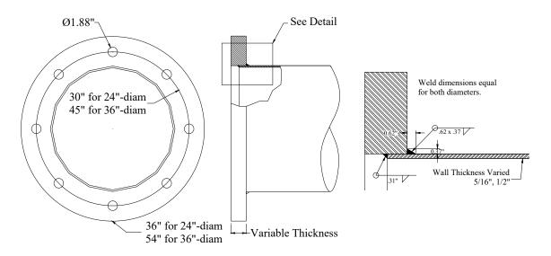
Figure 6.2: Connection Detail for Wall Thickness and Shaft Diameter Parametric Evaluation
