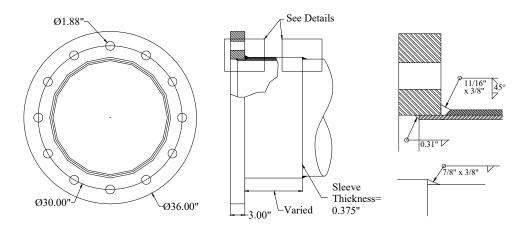
Figure 6.9: Socket External Collar Connection Detail
