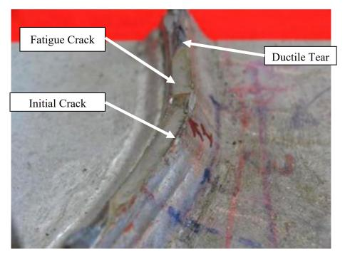
Figure 7.18: Bend 3 of Specimen 33-3-12-TX-VG-A
