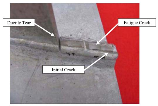
Figure 7.7: Close-up of Fracture Surface at Bend 5
