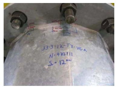
Figure 7.13: Specimen 33-3-12-TX-VG-A after Fatigue Testing
