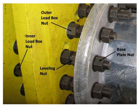
Figure 2.6: Double-Nut Connection and Nomenclature
