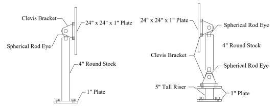
Figure 2.2: Test Setup End Supports High-mast Test (Rios, 2007)
