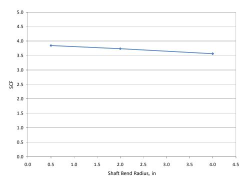
Figure 6.11: Results of Bend Radius Evaluation
