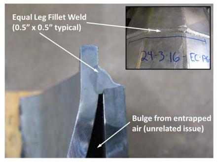
Figure 5.10: Typical Collar Weld in Pelco SEC Connection
