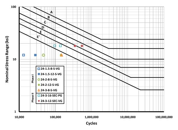
Figure 5.11: Socket Results for Phases I and II
