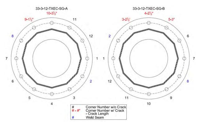
Figure 7.24: Crack Indications, Lengths, and Initial Orientation of External Collar Samples
