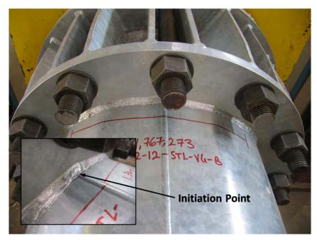
Figure 5.4: Stool Detail Fracture
