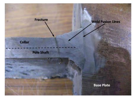
Figure 5.6: Section of Texas External Collar Connection
