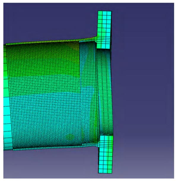
Figure 4.4: Bending of the Base Plate Connection (12-1.5R-WY)
