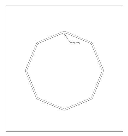
Figure 4.8: Typical Cross Section of Octagonal Mast arm
