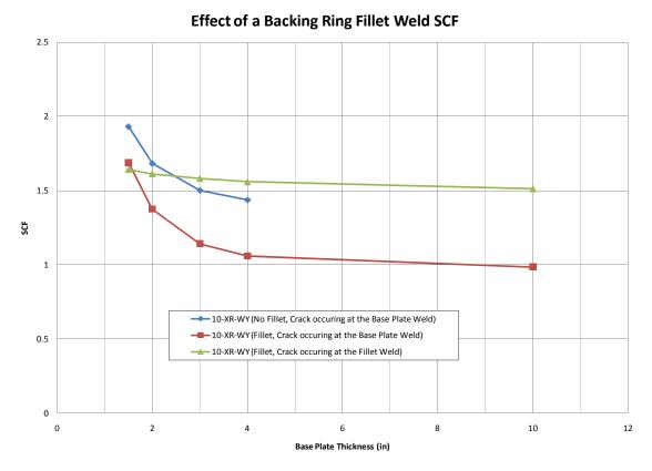
Figure 4.18: 10-XR-WY-FILLET (SCF versus Base Plate Thickness)
