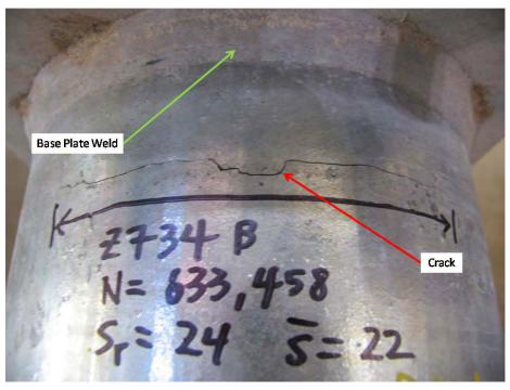
Figure 3.3: Typical Failure at a Backing Ring Fillet Weld
