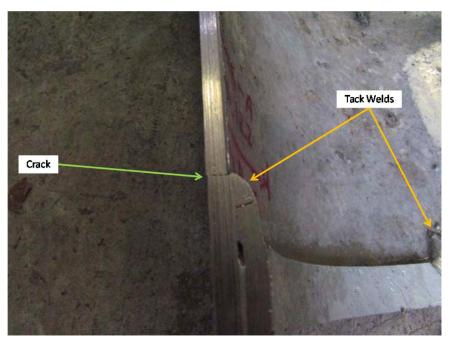
Figure 3.6: Cross Section of a Tack Weld Failure
