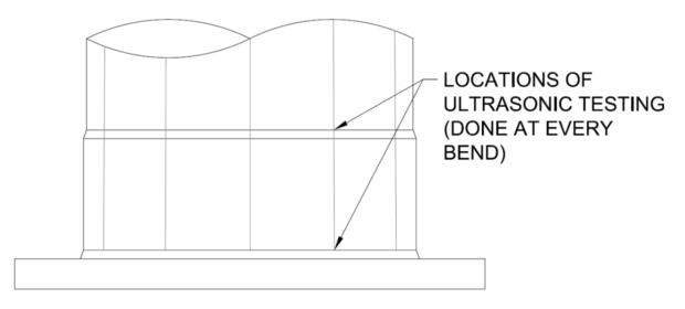
Figure 7.23: Locations Inspected Using Ultrasonic Testing on External Collar Samples
