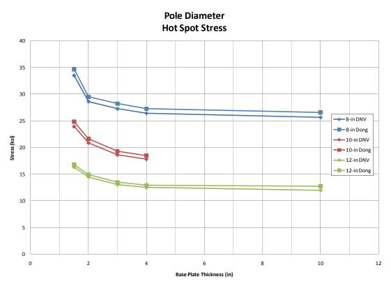
Figure 4.6: Mast arm Diameter Evaluation (Hot Spot Stress versus Base Plate Thickness)
