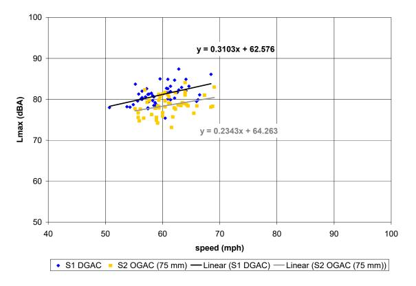
Figure C-15. Vehicle pass-by data, post-overlay, 4 months age; Site 1 (DGAC 30mm), Site 2 (OGAC 75mm). Automobiles (top), medium trucks (middle), and heavy trucks (bottom). Microphone location: distance 50 ft, height 15 ft.
