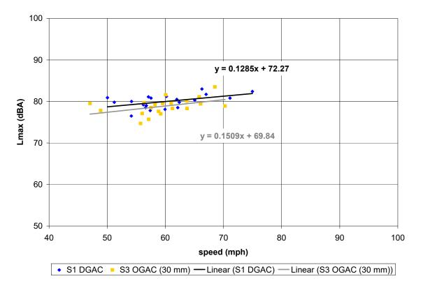
Figure C-29. (this and previous page) Vehicle pass-by data, post-overlay, 10 months age; Site 1 (DGAC 30mm), Site 3 (OGAC 30mm). Automobiles (top), medium trucks (middle), and heavy trucks (bottom). Microphone location: distance 50 ft, height 5 ft.
