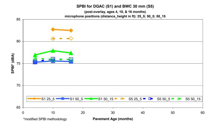
Figure D-4. SPBI\* values over time for pavement pair DGAC 30mm (S1) and BWC 30mm (S5). Overlay pavements aged 4, 10, and 16 months. Microphone locations: distance 7.5 m (25 ft), height 1.5 m (5 ft); distance 15 m (50 ft), height 1.5 m (5 ft); distance 15 m (50 ft), height 4.5 m (15 ft).
