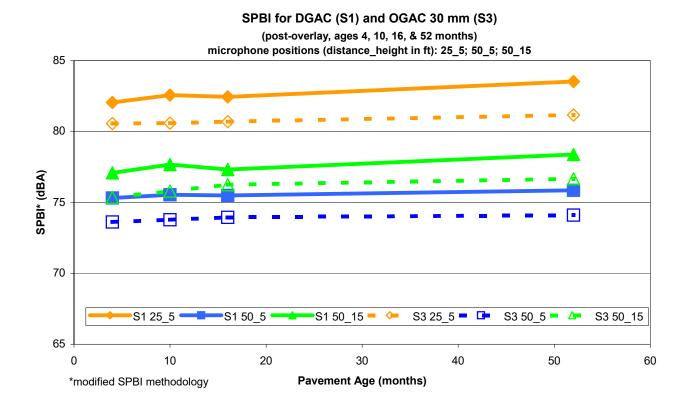
Figure D-2. SPBI\* values over time for pavement pair DGAC 30mm (S1) and OGAC 30mm (S3). Overlay pavements aged 4, 10, 16, and 52 months. Microphone locations: distance 7.5 m (25 ft), height 1.5 m (5 ft); distance 15 m (50 ft), height 1.5 m (5 ft); distance 15 m (50 ft), height 4.5 m (15 ft).
