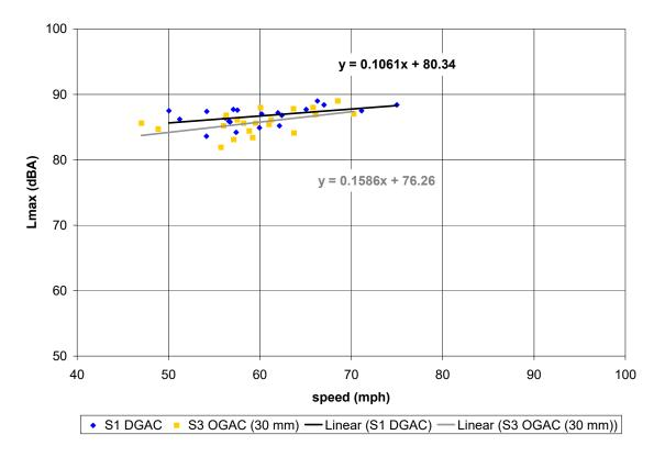
Figure C-28. (this and previous page) Vehicle pass-by data, post-overlay, 10 months age; Site 1 (DGAC 30mm), Site 3 (OGAC 30mm). Automobiles (top), medium trucks (middle), and heavy trucks (bottom). Microphone location: distance 25 ft, height 5 ft.
