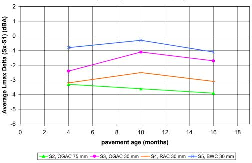
Test Vehicle (Subaru) 60 mph; microphone distance: 50 ft, height: 5 ft
