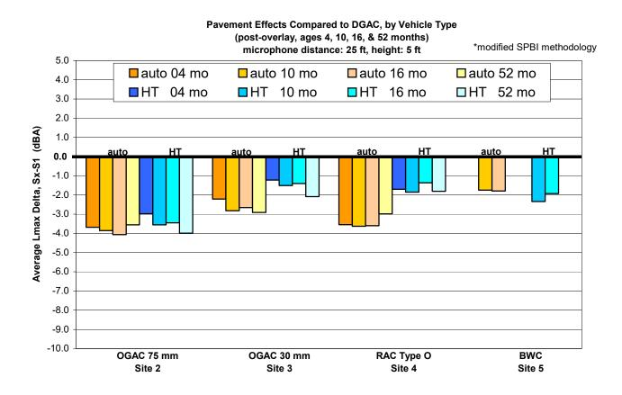
Figure E-1. Pavement effects compared to DGAC (Site x minus Site 1) for autos and heavy trucks using modified SPBI.\* Post-overlay results, all pavements, including DGAC, aged 4, 10, 16, and 52 months (limited data for BWC). Microphone location: distance 7.5 m (25 ft), height 1.5 m (5 ft).
