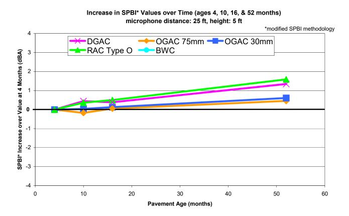
Figure 6. Increase in SPBI\* values over time, as compared to values at 4 months. Microphone location: distance 7.5 m (25 ft), height 1.5 m (5 ft).
