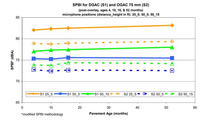
Figure D-1. SPBI\* values over time for pavement pair DGAC 30mm (S1) and OGAC 75mm (S2). Overlay pavements aged 4, 10, 16, and 52 months. Microphone locations: distance 7.5 m (25 ft), height 1.5 m (5 ft); distance 15 m (50 ft), height 1.5 m (5 ft); distance 15 m (50 ft), height 4.5 m (15 ft).
