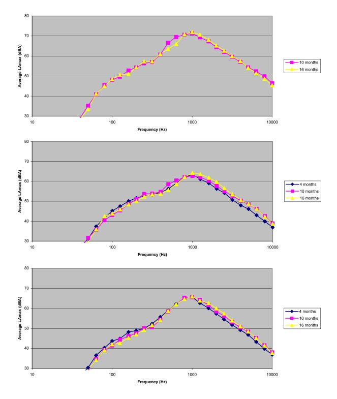
Figure E-23. Spectral data for automobiles; post-overlay results for Site 5 (BWC 30 mm); all ages measured. Microphone location: distance 25 ft, height 5 ft (top); microphone location: distance 50 ft, height 5 ft (middle); microphone location: distance 50 ft, height 15 ft (bottom).
