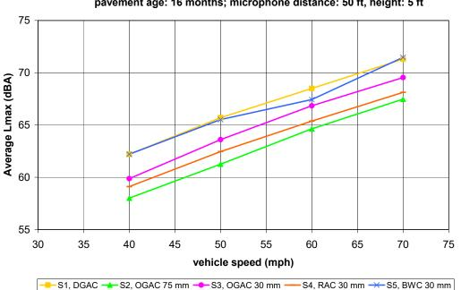
Test Vehicle (Subaru) pavement age: 16 months; microphone distance: 50 ft, height: 5 ft
