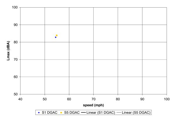
Figure C-12. (this and previous page) Vehicle pass-by data, pre-overlay; Site 1 (DGAC), Site 5 (DGAC). Automobiles (top), medium trucks (middle), and heavy trucks (bottom). Microphone location: distance 50 ft, height 15 ft.
