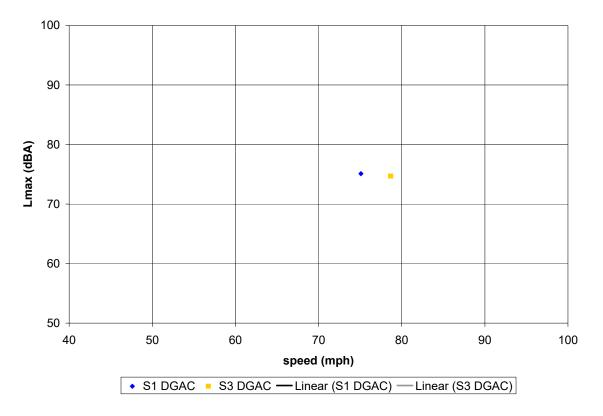
Figure C-6. (this and previous page) Vehicle pass-by data, pre-overlay; Site 1 (DGAC), Site 3 (DGAC). Automobiles (top), medium trucks (middle), and heavy trucks (bottom). Microphone location: distance 50 ft, height 15 ft.
