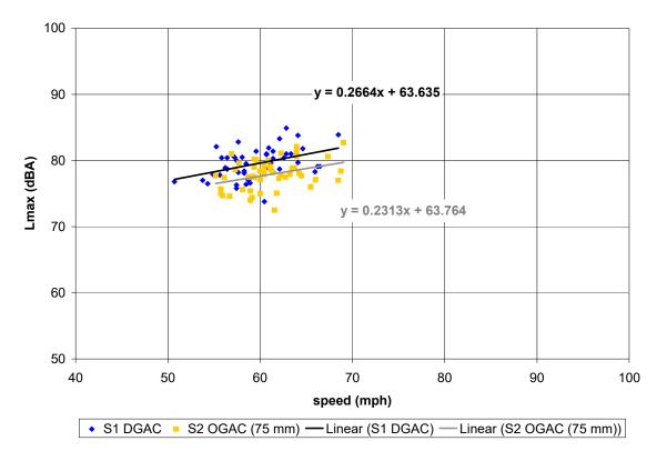
Figure C-14. (this and previous page) Vehicle pass-by data, post-overlay, 4 months age; Site 1 (DGAC 30mm), Site 2 (OGAC 75mm). Automobiles (top), medium trucks (middle), and heavy trucks (bottom). Microphone location: distance 50 ft, height 5 ft.
