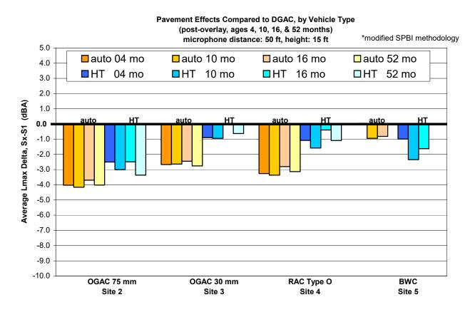
Figure E-3. Pavement effects compared to DGAC (Site x minus Site 1) for autos and heavy trucks using modified SPBI.\* Post-overlay results, all pavements, including DGAC, aged 4, 10, 16, and 52 months (limited data for BWC). Microphone location: distance 15 m (50 ft), height 4.5 m (15 ft).
