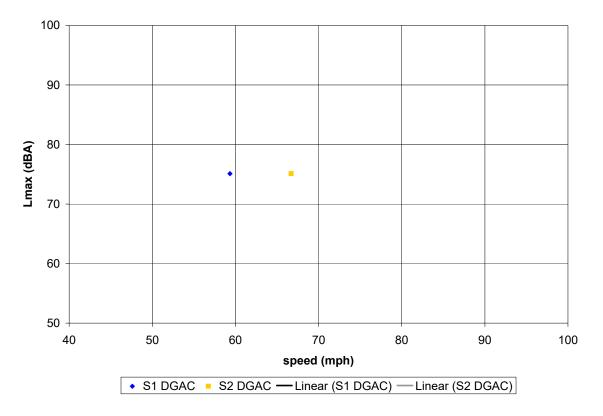
Figure C-3. (this and previous page) Vehicle pass-by data, pre-overlay; Site 1 (DGAC), Site 2 (DGAC). Automobiles (top), medium trucks (middle), and heavy trucks (bottom). Microphone location: distance 50 ft, height 15 ft.
