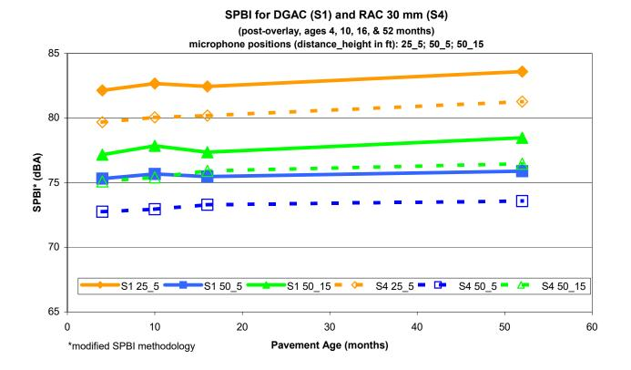
Figure D-3. SPBI\* values over time for pavement pair DGAC 30mm (S1) and RAC Type O 30mm (S4). Overlay pavements aged 4, 10, 16, and 52 months. Microphone locations: distance 7.5 m (25 ft), height 1.5 m (5 ft); distance 15 m (50 ft), height 1.5 m (5 ft); distance 15 m (50 ft), height 4.5 m (15 ft).
