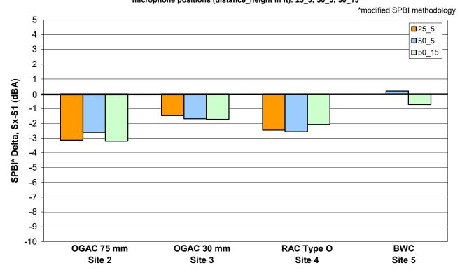
Pavement Effects Compared to DGAC (post-overlay, age ~4 mo) microphone positions (distance\_height in ft): 25\_5; 50\_5; 50\_15
