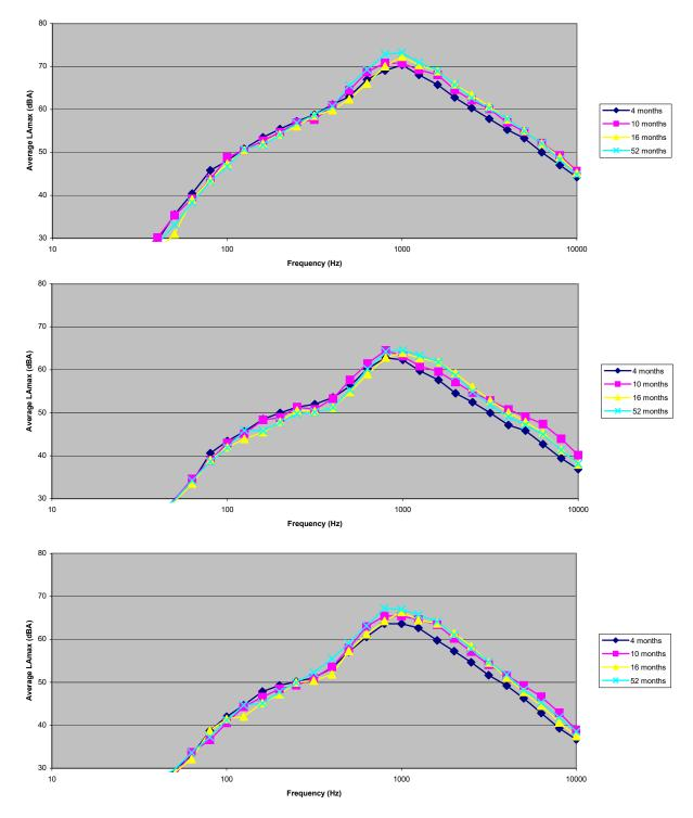
Figure E-19. Spectral data for automobiles; post-overlay results for Site 1 (DGAC 30 mm); all ages measured. Microphone location: distance 25 ft, height 5 ft (top); microphone location: distance 50 ft, height 5 ft (middle); microphone location: distance 50 ft, height 15 ft (bottom).
