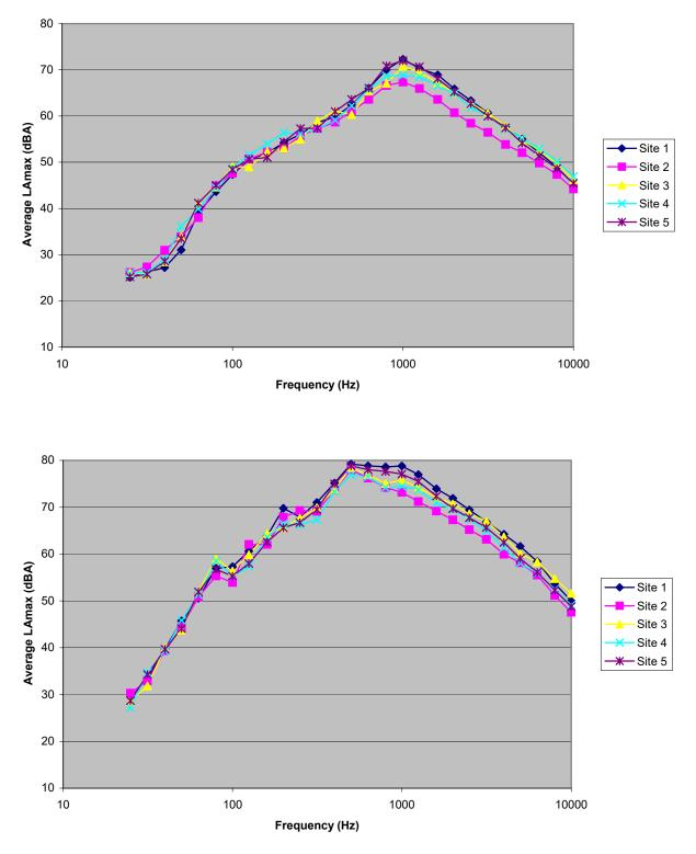
Figure E-12. Spectral data for automobiles (top) and heavy trucks (bottom) on four different pavement types. Post-overlay results, all pavements aged 16 months. Microphone location: distance 25 ft, height 5 ft.
