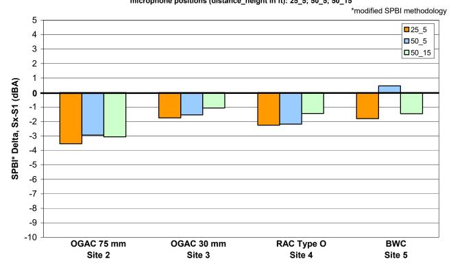
Pavement Effects Compared to DGAC (post-overlay, age ~16 mo) microphone positions (distance\_height in ft): 25\_5; 50\_5; 50\_15
