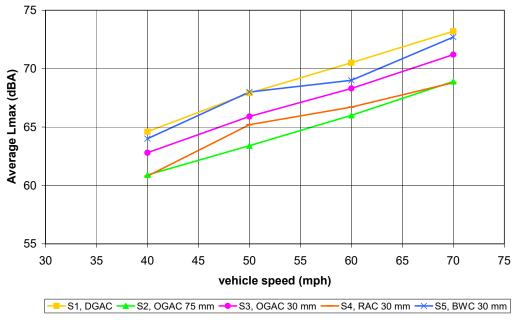
Figure F-3. Test vehicle average L<sub>AFmx</sub> values for pavement aged 16 months, multiple speeds. Microphone position: (top) distance 15 m (50 ft), height 1.5 m (5 ft); (bottom) distance 15 m (50 ft), height 4.5 m (15 ft). Site bias removed.
