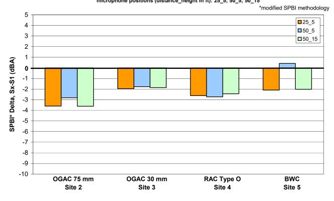
Pavement Effects Compared to DGAC (post-overlay, age ~10 mo) microphone positions (distance\_height in ft): 25\_5; 50\_5; 50\_15
