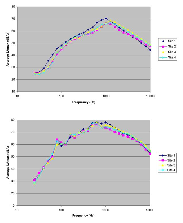
Figure E-4. Spectral data for automobiles (top) and heavy trucks (bottom) on four different pavement types. Post-overlay results, all pavements aged 4 months. Microphone location: distance 25 ft, height 5 ft.
