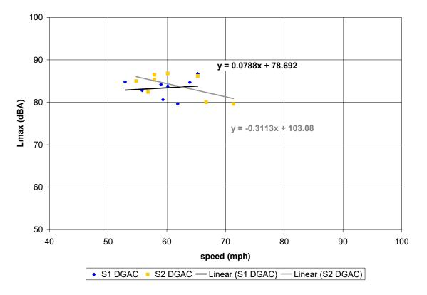
Figure C-1. (this and previous page) Vehicle pass-by data, pre-overlay; Site 1 (DGAC), Site 2 (DGAC). Automobiles (top), medium trucks (middle), and heavy trucks (bottom). Microphone location: distance 25 ft, height 5 ft.
