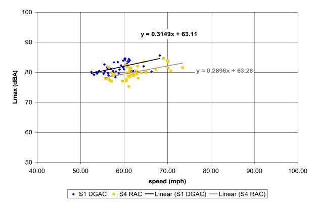
Figure C-45. (this and previous page) Vehicle pass-by data, post-overlay, 16 months age; Site 1 (DGAC 30mm), Site 4 (RAC Type O 30mm). Automobiles (top), medium trucks (middle), and heavy trucks (bottom). Microphone location: distance 50 ft, height 15 ft.
