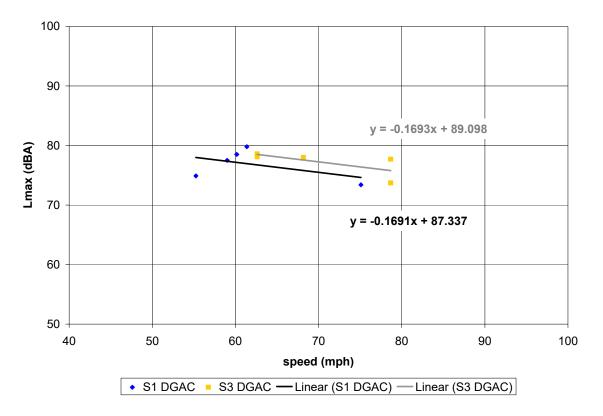
Figure C-5. (this and previous page) Vehicle pass-by data, pre-overlay; Site 1 (DGAC), Site 3 (DGAC). Automobiles (top), medium trucks (middle), and heavy trucks (bottom). Microphone location: distance 50 ft, height 5 ft.
