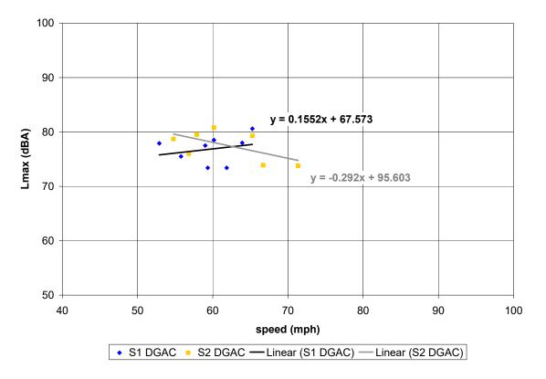
Figure C-2. (this and previous page) Vehicle pass-by data, pre-overlay; Site 1 (DGAC), Site 2 (DGAC). Automobiles (top), medium trucks (middle), and heavy trucks (bottom). Microphone location: distance 50 ft, height 5 ft.
