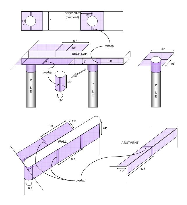
Figure 2. Locations of surface modifications on highway structures with pile bents and pier walls. Dimensions x, y, and z varied depending on the site. (Diagram not to scale)
