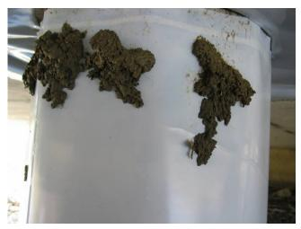
Figure 7. Mud sliding down surface of PTFE surface modification on column.
