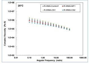
Figure 4.24: Phase 2, Mix Design #1: Viscosity at 25°C at zero aging (loose mix).
