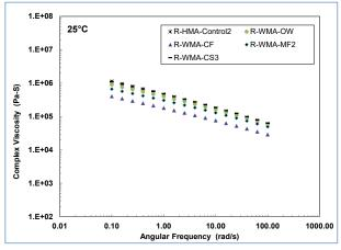
Figure 4.28: Phase 2, Mix Design #2: Viscosity at 25°C at zero aging.
