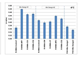
Figure 4.59: Phase 2: Comparison of m-values at -6° C after 14 months field aging.
