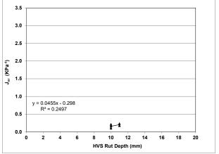
Figure 4.51: Phase 2, Mix Design #2: Non-recoverable compliance versus HVS rut depth.
