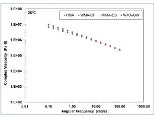
Figure 4.16: Phase 1: Viscosity at 25°C after 48 months.
