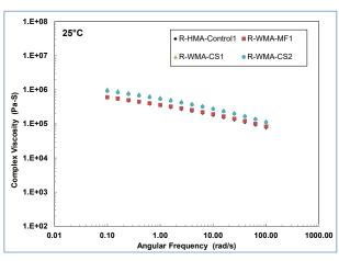
Figure 4.26: Phase 2, Mix Design #1: Viscosity at 25°C after 14 months.
