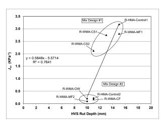
Figure 4.49: Phase 2: Non-recoverable compliance versus HVS rut depth.
