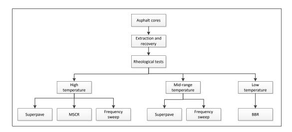
Figure 3.1: Schematic of experimental plan for binder testing.
