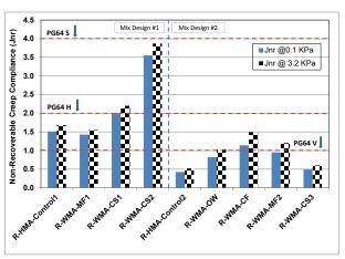
Figure 4.6: Conventional binder: non-recoverable creep compliance.
