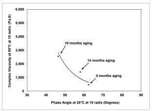
Figure 4.31: Phase 1: Viscosity-phase angle relationship with aging kinetics.
