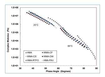
Figure 4.12: Phase 1: Black diagram for binders after 52 months.
