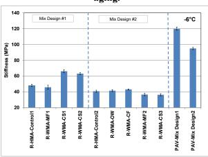
Figure 4.58: Phase 2: Comparison of stiffness values at -6°C after 14 months field aging.
