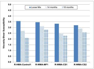
Figure 4.3: Conventional binder: VSS at different aging times.
