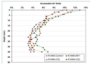
Figure 4.43: Phase 2: Accessible air-void content versus depth for control mixes.
