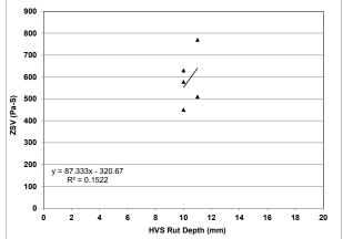
Figure 4.54: Phase 2, Mix Design #1: ZSV versus HVS rut depth.
