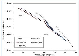
Figure 4.10: Phase 1: Black diagram for binders at zero aging (loose mix). Figure 4.11: Phase 1: Black diagram for binders after 48 months.
