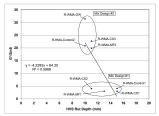
Figure 4.48: Phase 2: G\*/sin\u00e3 at 64\u00a3C versus HVS rut depth.
