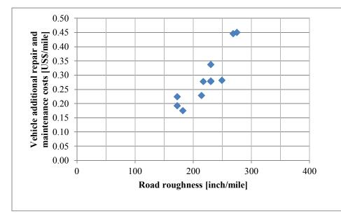
Figure 5.10: Potential increase in vehicle maintenance and repair cost due to bad roads.
