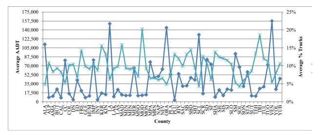
Figure 4.5: AADT and percentage trucks data for Caltrans counties ( $\neq$ =AADT;  $\times$  = % Trucks).
