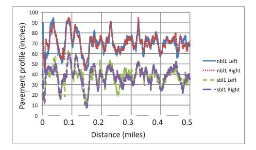
Figure 3.1: Example of four typical road profiles.
