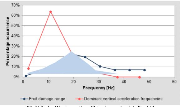
[[lt: (1) Hz should be in parentheses (Hz), not square brackets. Bn: stet]] Figure 5.12: Comparison between dominant frequencies experienced by fruit cargo and the vibration range that results in damage.
