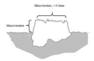
Figure 3.2: Definition of macrotexture and microtexture of pavement surfacing aggregate (6).
