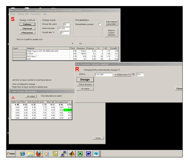
Figure E.1: Screen shot of R-Value design using CalME
