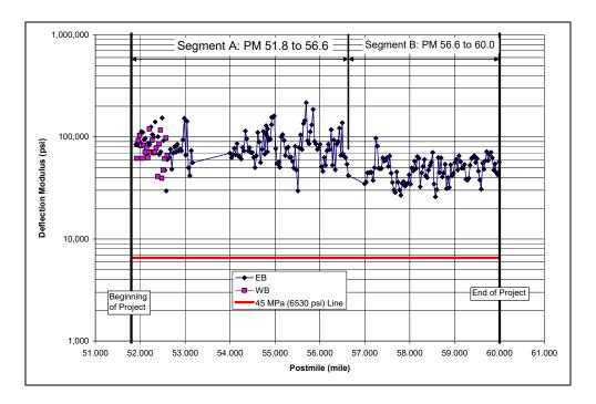
Figure D.1: Subgrade Deflection Modulus.
