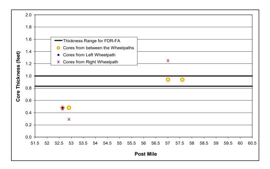
Figure C.2: HMA thickness summary from cores for westbound lane.
