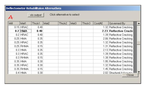
Figure E.3: Partial list of alternatives for mill and overlay option from CalME.
