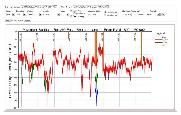
Figure C.5: Screenshot from PMS GPR/Core viewing tool. (note that pavement layer depth is in centimeters [30 cm = 1 ft]).
