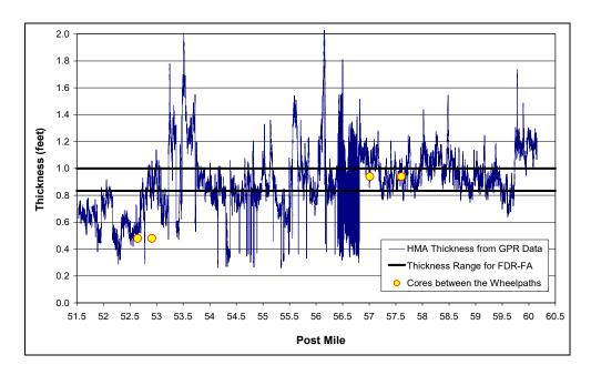
Figure C.4: Comparison of GPR and core thicknesses for westbound lane.
