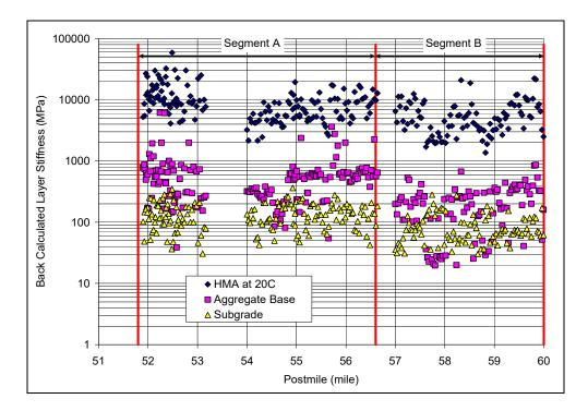
Figure D.2: Backcalculated layer stiffness and uniform subsection boundaries.
