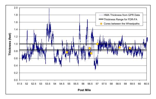
Figure C.3: Comparison of GPR and core thicknesses for eastbound lane.
