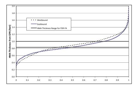
Figure 2.5: Cumulative distribution plot of HMA thickness from GPR.
