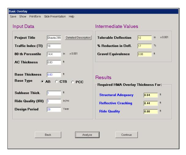
Figure E.4: Input screen for *CalAC* (changing subbase thickness to 0 ft did not change the result).
