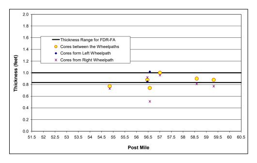
Figure C.1: HMA thickness summary from cores for eastbound lane.
