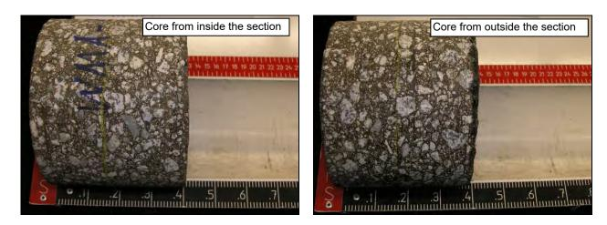
Figure 4.27: 605FD: Cores for moisture content determination.
