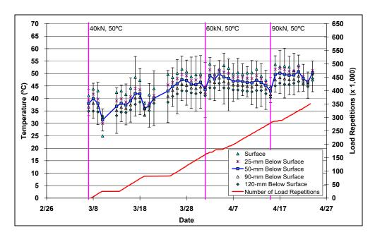
Figure 4.36: 606FD: Daily average temperatures at pavement surface and various depths.
