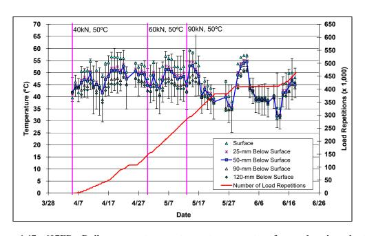
Figure 4.47: 607FD: Daily average temperatures at pavement surface and various depths.
