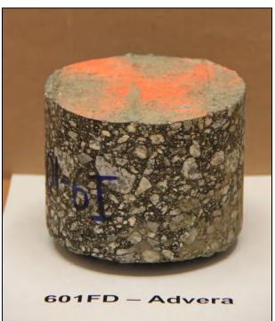
Figure 5.2: 600FD: Core from Trafficked Area.
