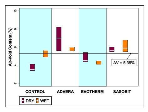
Figure 6.7: Air-void contents of flexural frequency sweep specimens (dry and wet).
