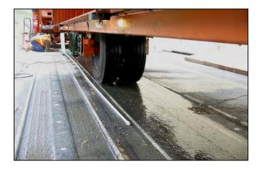
Figure 3.6: Water flow across test section during trafficking.
