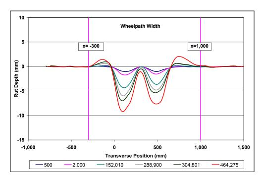
Figure 4.48: 607FD: Profilometer cross section at various load repetitions.
