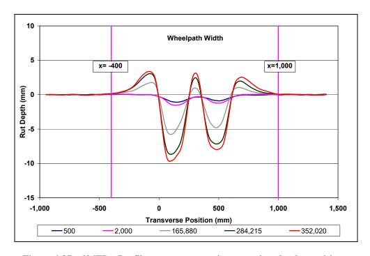
Figure 4.37: 606FD: Profilometer cross section at various load repetitions.
