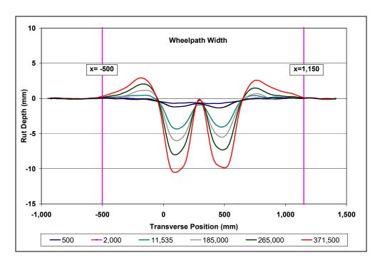
Figure 4.8: 604FD: Profilometer cross section at various load repetitions.
