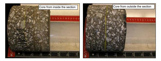
Figure 4.52: 607FD: Cores for moisture content determination.
