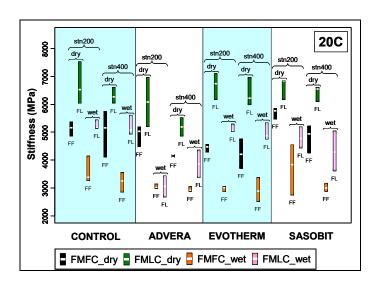
Figure 6.22: Initial stiffness comparison between FMFC and FMLC fatigue tests.
