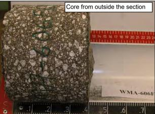
Figure 4.41: 606FD: Cores for moisture content determination.
