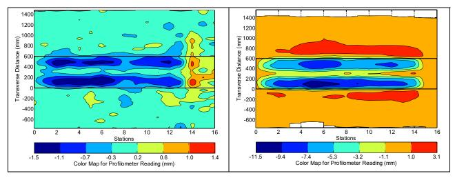
Figure 4.51: 607FD: Contour plot of permanent surface deformation at start and end of test.
