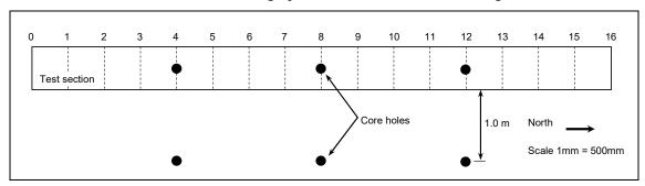
Figure 4.12: Location of cores for moisture content determination.
