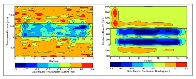
Figure 4.11: 604FD: Contour plot of permanent surface deformation at start and end of test.
