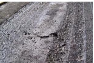
Figure 4.29: 605FD: Cracks in wheelpaths during testing.
