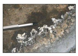
Figure 4.14: 604FD: Crystallized salt on edges of wheelpaths during testing.
