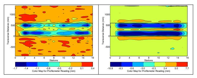
Figure 4.40: 606FD: Contour plot of permanent surface deformation at start and end of test. (Note that scales are different.)
