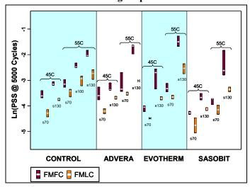
Figure 6.20: Permanent shear strain comparison between FMFC and FMLC shear tests.
