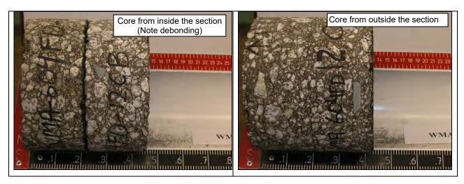
Figure 4.13: 604FD: Cores for moisture content determination.
