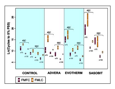
Figure 6.21: Cycles to 5% permanent shear strain comparison between FMFC and FMLC shear tests.
