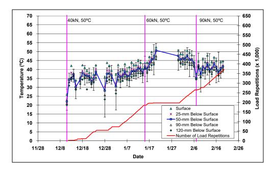
Figure 4.7: 604FD: Daily average temperatures at pavement surface and various depths.
