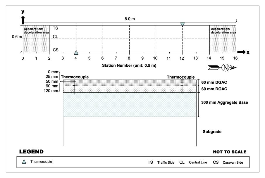
Figure 3.2: Phase 2 test section layout and thermocouple locations.
