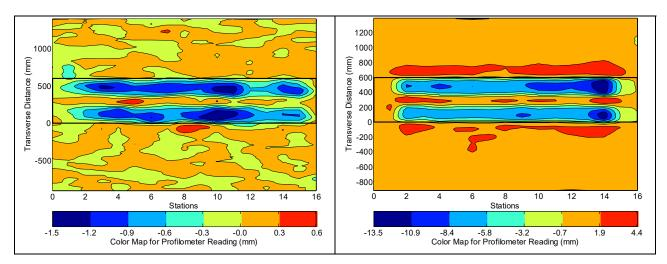
Figure 4.26: 605FD: Contour plot of permanent surface deformation at start and end of test. (Note that scales are different.)
