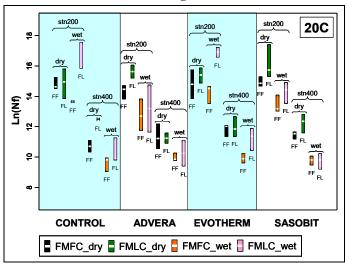
Figure 6.24: Fatigue life comparison between FMFC and FMLC fatigue tests.
