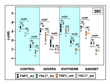
Figure 6.26: Comparison of fatigue life after air-void content correction.
