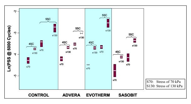
Figure 6.4: Summary boxplots of cumulative permanent shear strain at 5,000 cycles.
