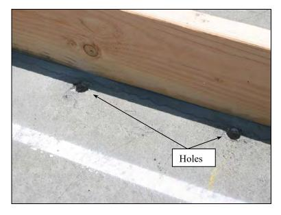
Figure 3.4: Soaking dam and presoaking holes.
