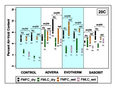
Figure 6.18: Air-void content comparison between FMFC and FMLC fatigue specimens.
