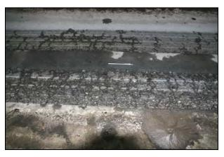
Figure 4.15: 604FD: Cracks in wheelpaths during testing.
