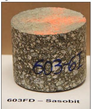
Figure 5.4: 602FD: Core from Trafficked Area. Figure 5.5: 603FD: Core from Trafficked Area.
