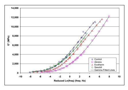
Figure 6.12: Flexural complex modulus  $(E^*)$  master curves (dry).
