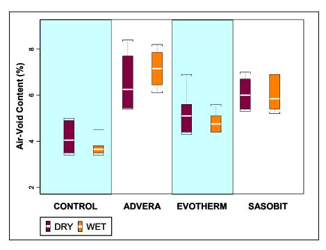
Figure 6.6: Air-void contents of fatigue beam specimens (dry and wet).
