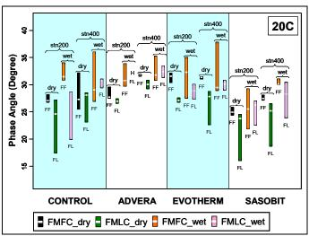
Figure 6.23: Phase angle comparison between FMFC and FMLC fatigue tests.
