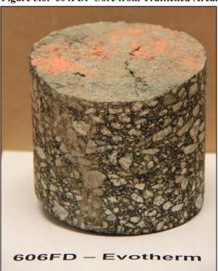
Figure 5.7: 605FD: Core from Trafficked Area.
