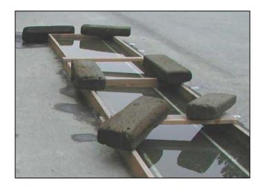
Figure 3.5: Soaking dam with water.
