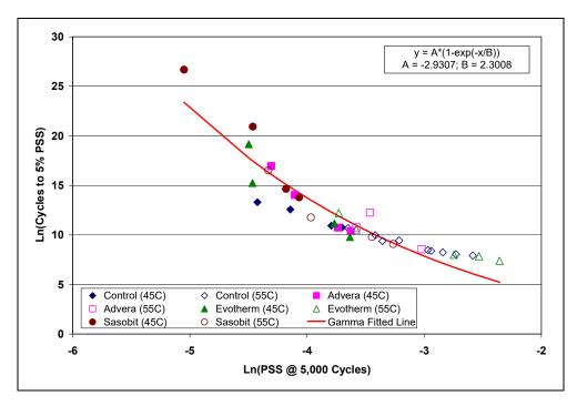
Figure 6.5: Cycles to 5% permanent shear strain versus permanent shear strain after 5,000 cycles.
