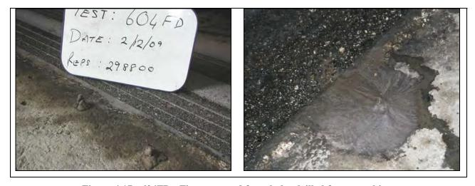
Figure 4.17: 604FD: Fines pumped from holes drilled for presoaking.
