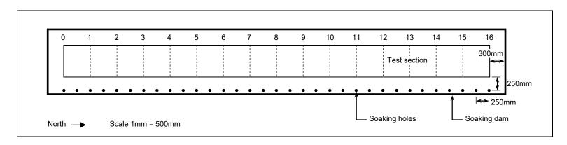
Figure 3.3: Location of presoaking dam and soak holes.
