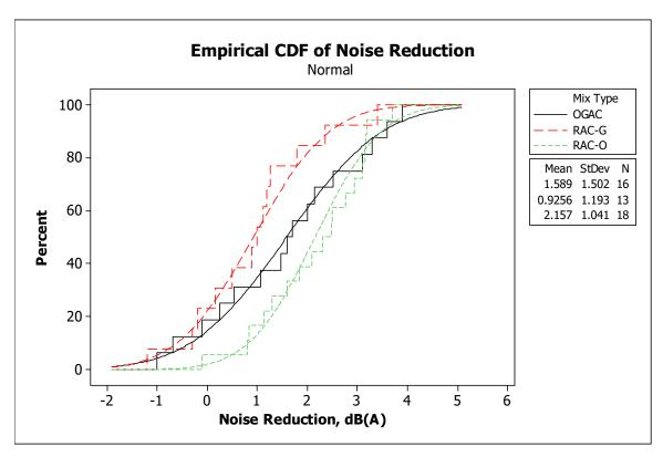
Figure 7: Cumulative distribution function of noise reduction of OGAC, RAC-O, and RAC-G mixes compared to DGAC (104 dB(A) average across all ages) across an eight-year range of ages (positive value indicates a reduction in noise).
