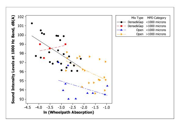
Figure 9: Sound intensity levels at 1,000 Hz band versus the absorption values for different mix types and different macrotexture values.
