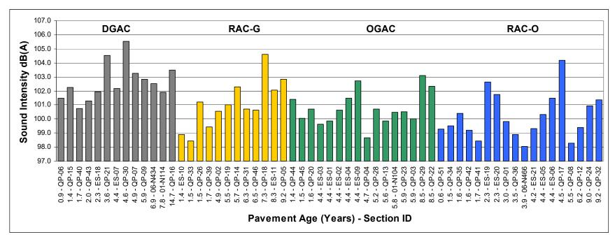
Figure A3: Second-year OBSI (SRTT tire) organized by material type and then sorted by increasing age (age in years since construction shown in front of section number on x-axis).
