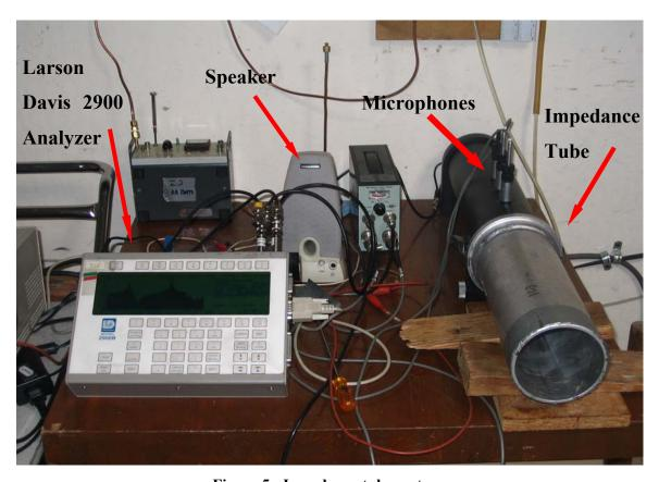
Figure 5: Impedance tube system.
