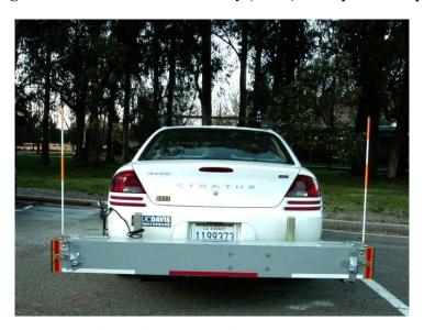
Figure 4: Laser profilometer beam.
