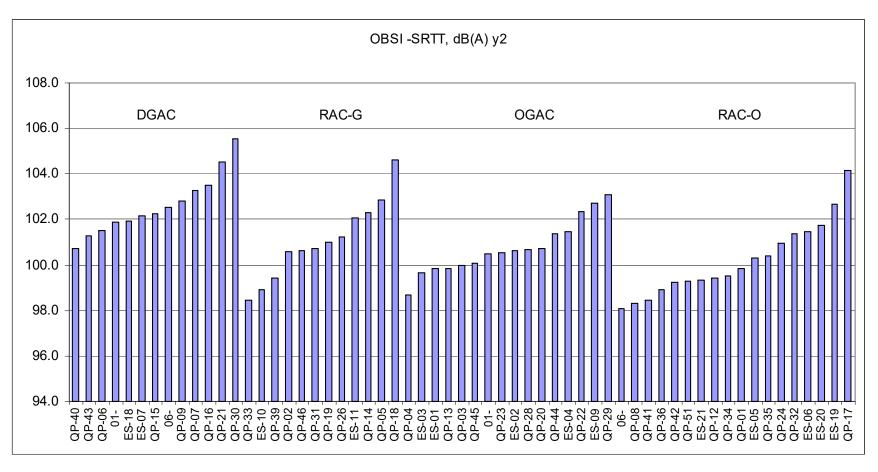
Figure A2. Second-year OBSI (SRTT tire) organized by material type and then sorted by increasing noise level.
