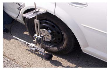
Figure 3: On-board sound intensity (OBSI) microphone setup.
