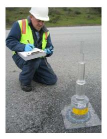
Figure 1: Falling-head permeameter.
