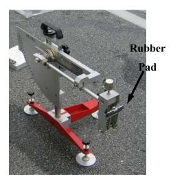
Figure 2: British Pendulum skid-resistance tester.
