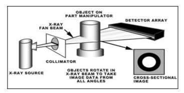
Figure 6: Computed tomography (CT) scanner (5).
